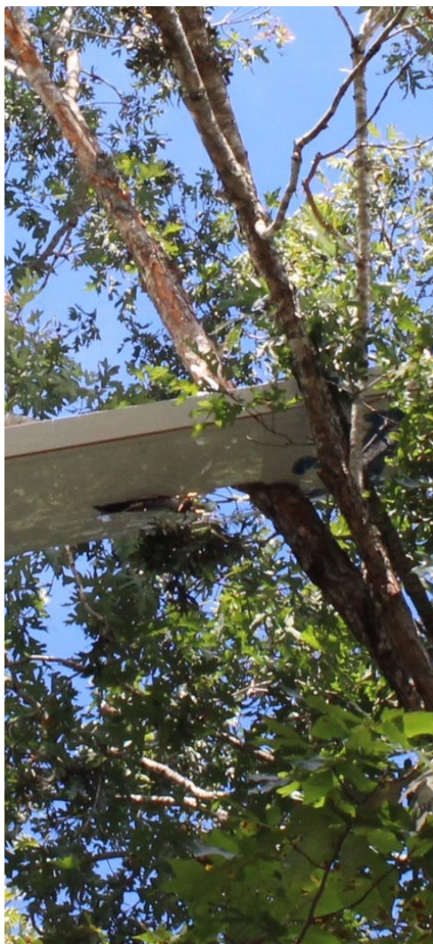
Photograph 2 - Right Wing Damage (Courtesy of FAA)
