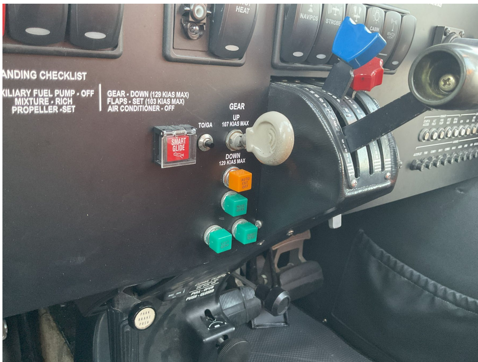
Photograph 4 - Gear Handle Up Position (Courtesy of FAA)
