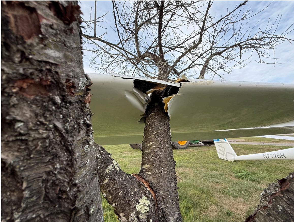
Photograph 3 - Right Wing Damage, Impact with Tree (Courtesy of FAA)
