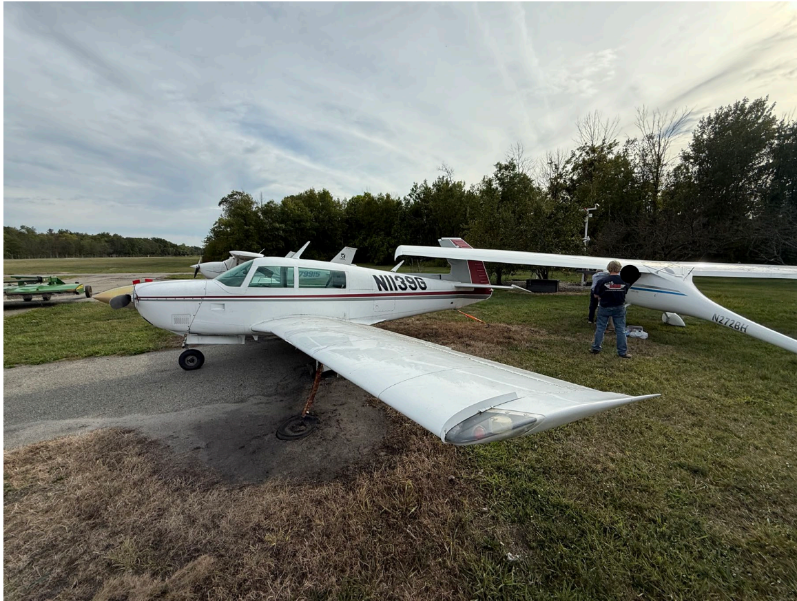
Photograph 2 - Left Wing Impact with Parked Aircraft (Courtesy of FAA)
