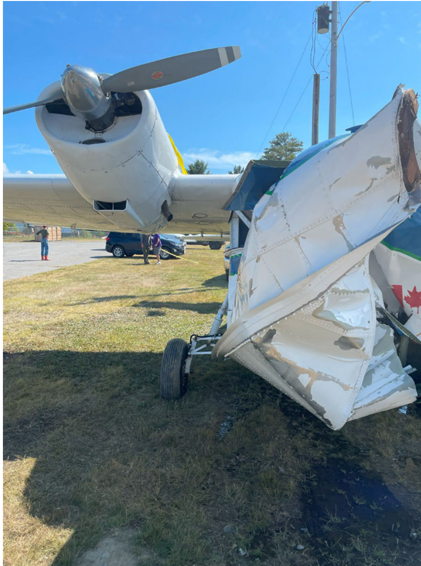
Photograph 5 - Right forward fuselage and hull accident damage (Courtesy of FAA)
