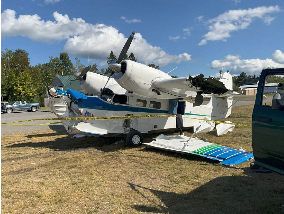
Photograph 1 - Airplane, postaccident with separated left wing (Courtesy of FAA)
