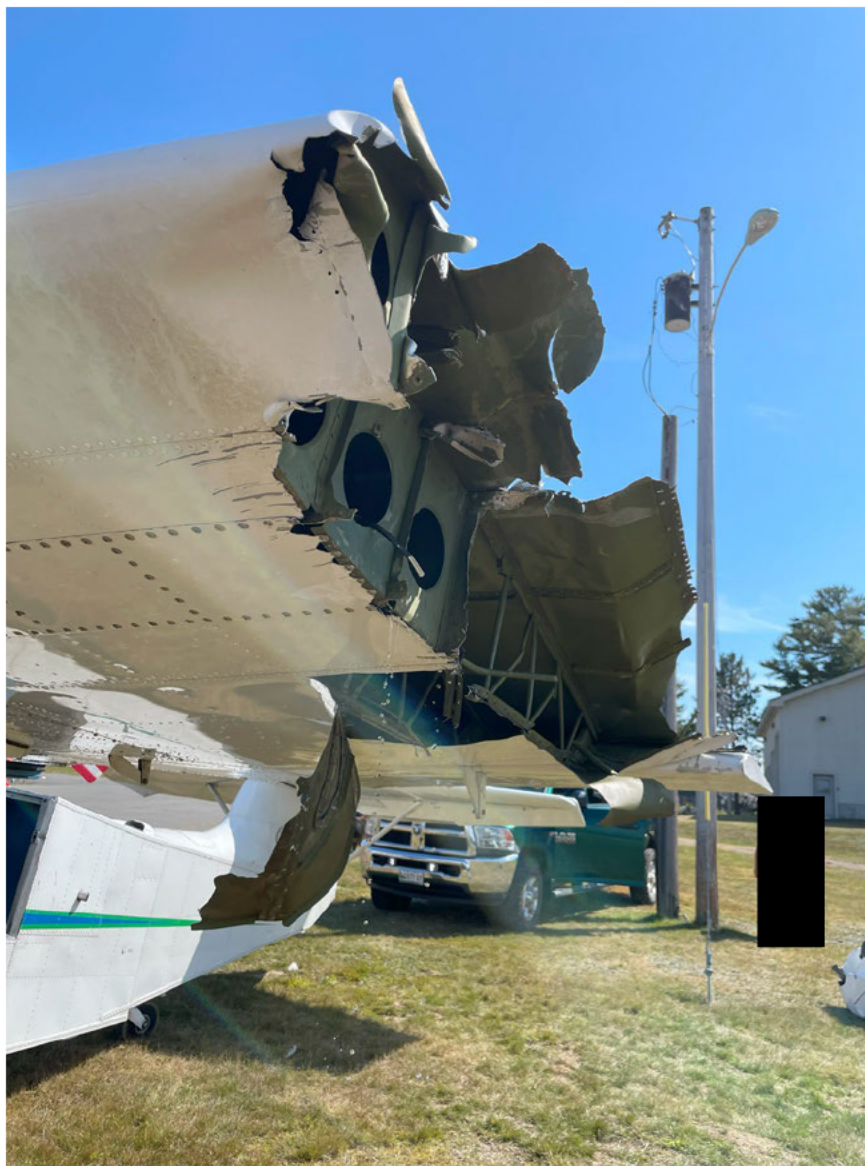
Photograph 3 - Left wing separation accident damage (Courtesy of FAA)
