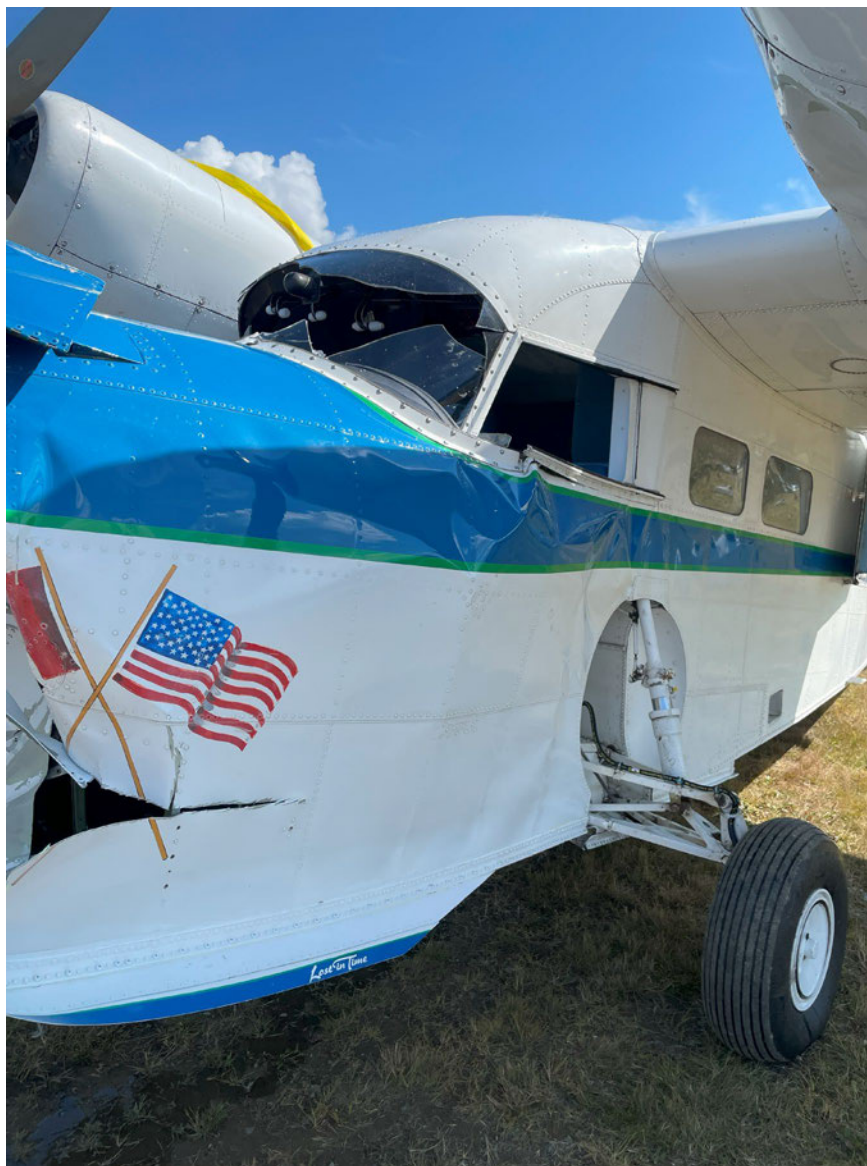
Photograph 4 - Left forward fuselage accident damage (Courtesy of FAA)
