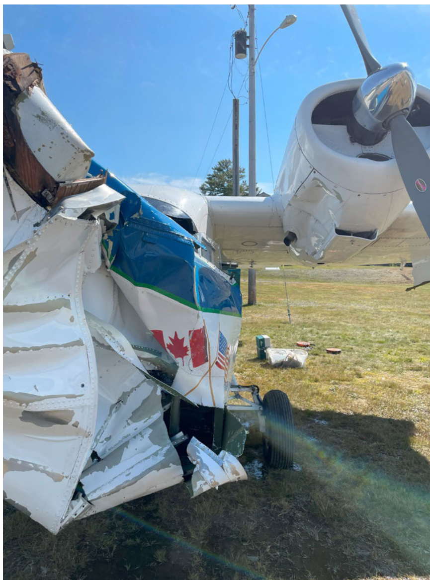
Photograph 2 - Left forward fuselage accident damage with breached hull (Courtesy of FAA)
