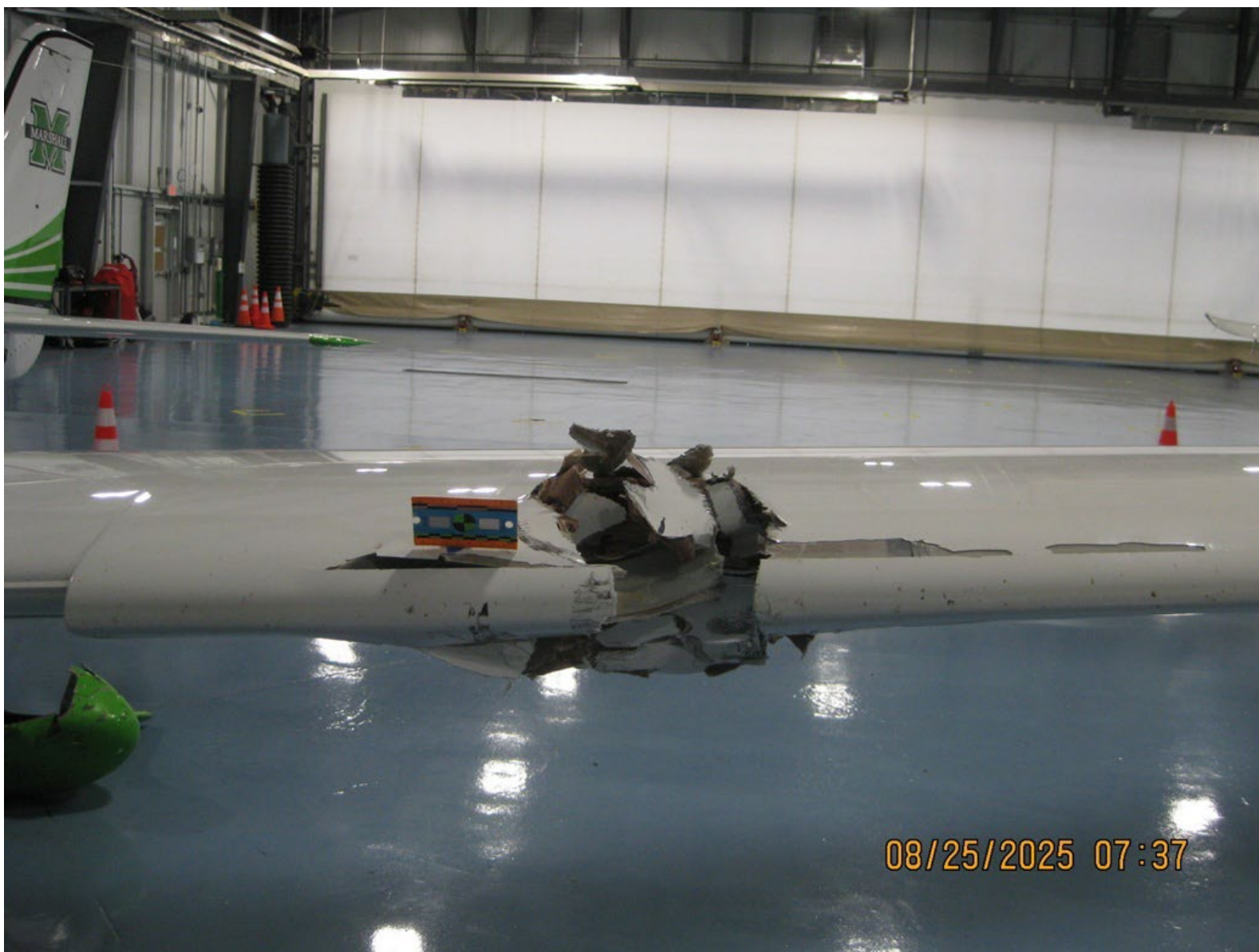
Photograph 1 - Left Wing Damage (Courtesy of FAA)
