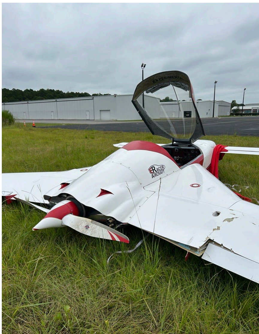
Photograph 1 - View of damage right wing. (Courtesy of FAA)
