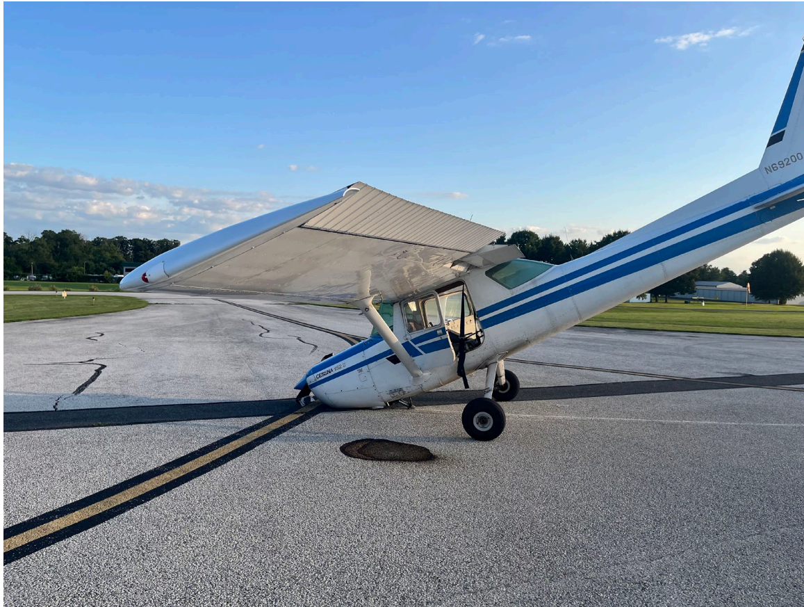
Photograph 1 - Left side of airplane with nose wheel collapse at accident site (Courtesy of FAA)
