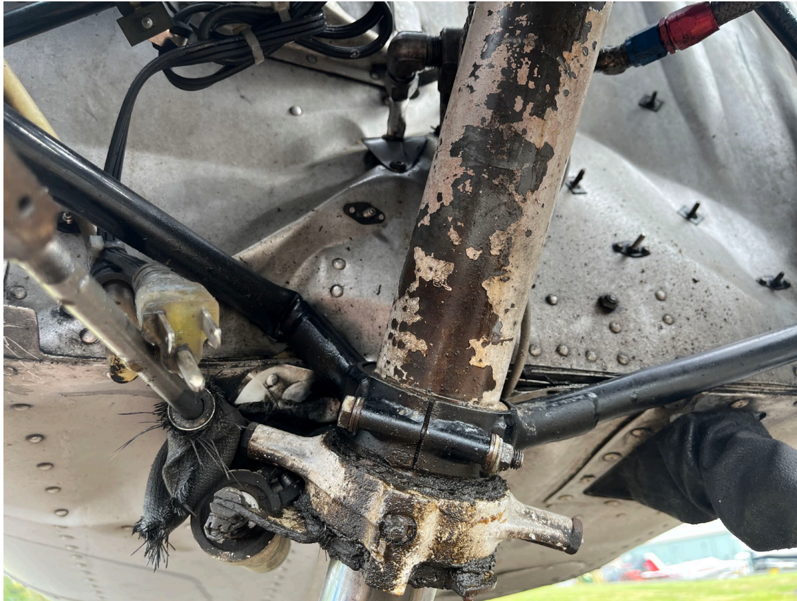
Photograph 2 - Damaged engine mount and collapsed nose wheel strut (Courtesy of FAA)
