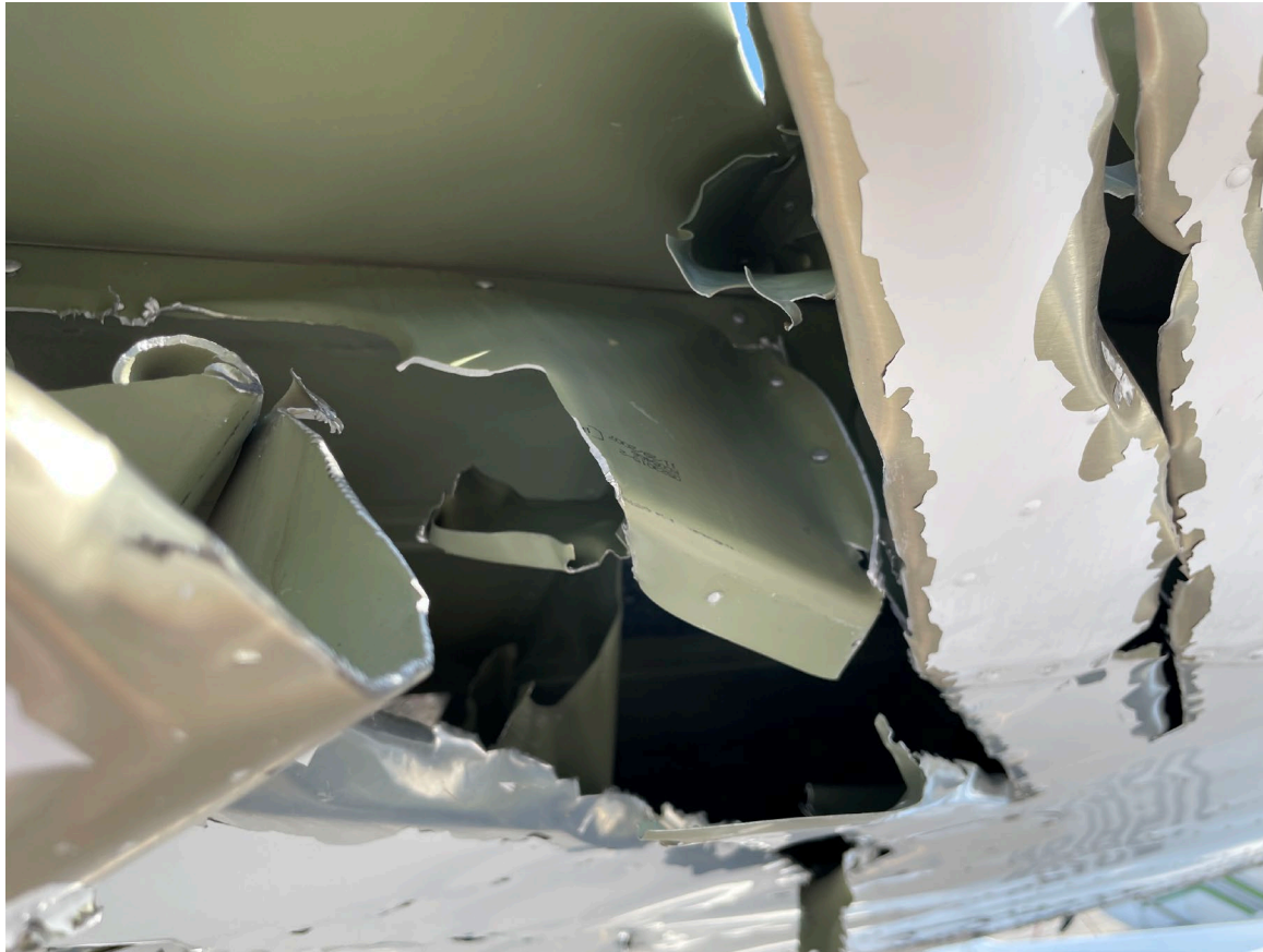
Photograph 4 - Close up View Showing Right Wing Spar Damage to N6185U (Courtesy of FAA)
