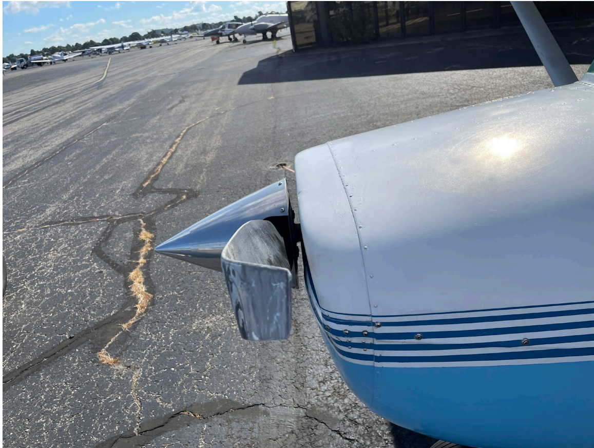
Photograph 5 - View of Damage to One Propeller Blade of N22998 (Courtesy of FAA)
