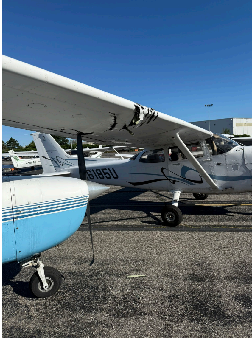
Photograph 3 - View of Resting Position of Both Airplanes (Courtesy of FAA). Note the Damage to the Right Wing of N6185U
