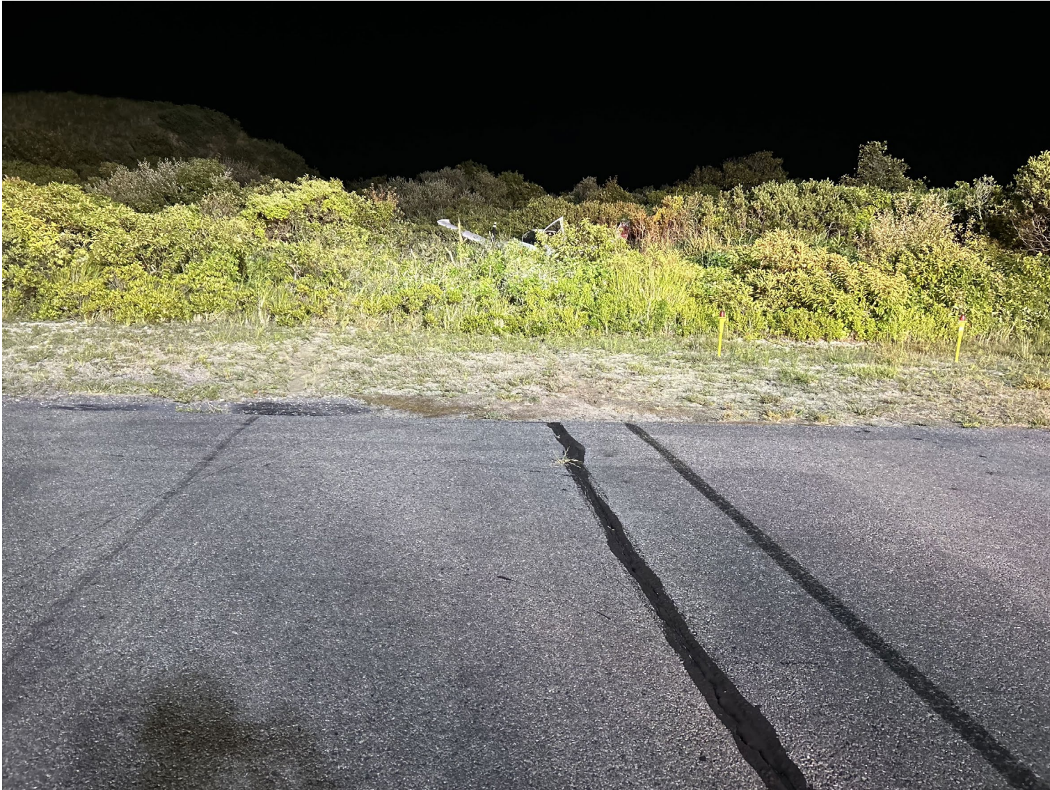
Photograph 2 - Skid Marks from the Braking Application (Courtesy of FAA)
