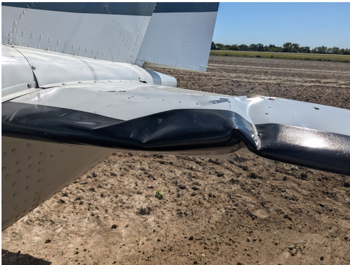
Photograph 2 - Left horizontal stabilizer accident damage (Courtesy of FAA)
