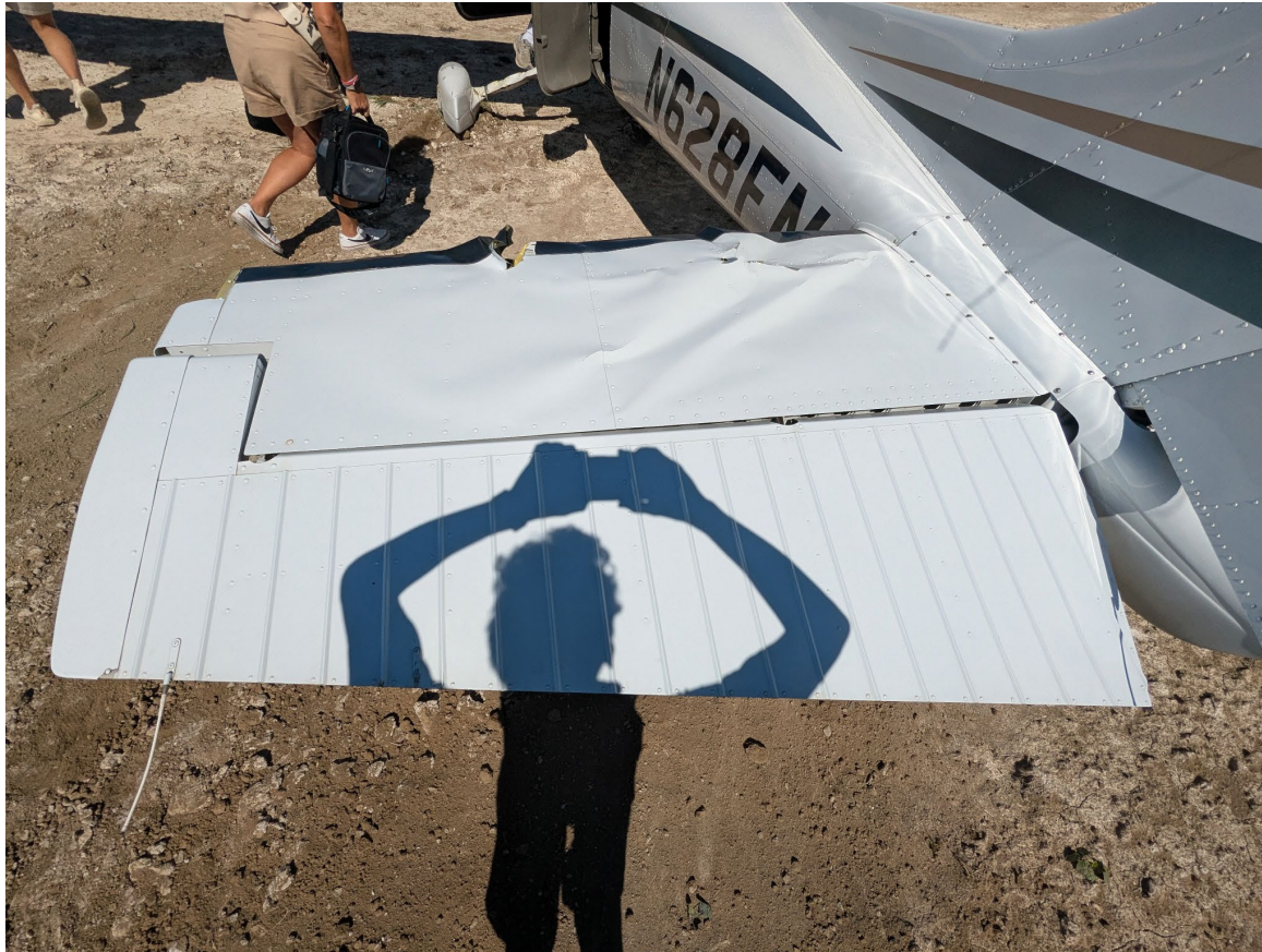
Photograph 3 - Left horizontal stabilizer accident damage (Courtesy of FAA)
