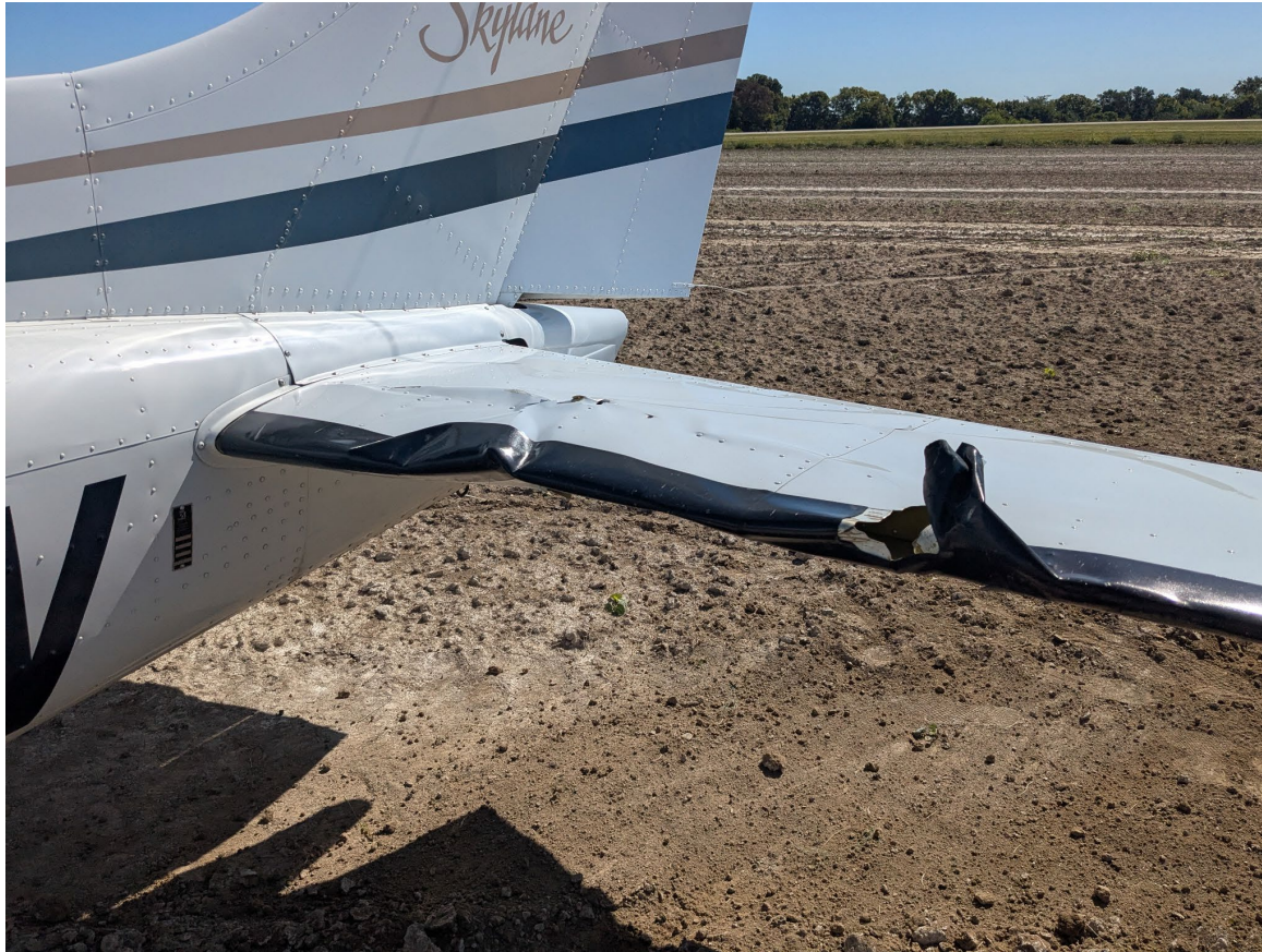
Photograph 1 - Left horizontal stabilizer accident damage (Courtesy of FAA)
