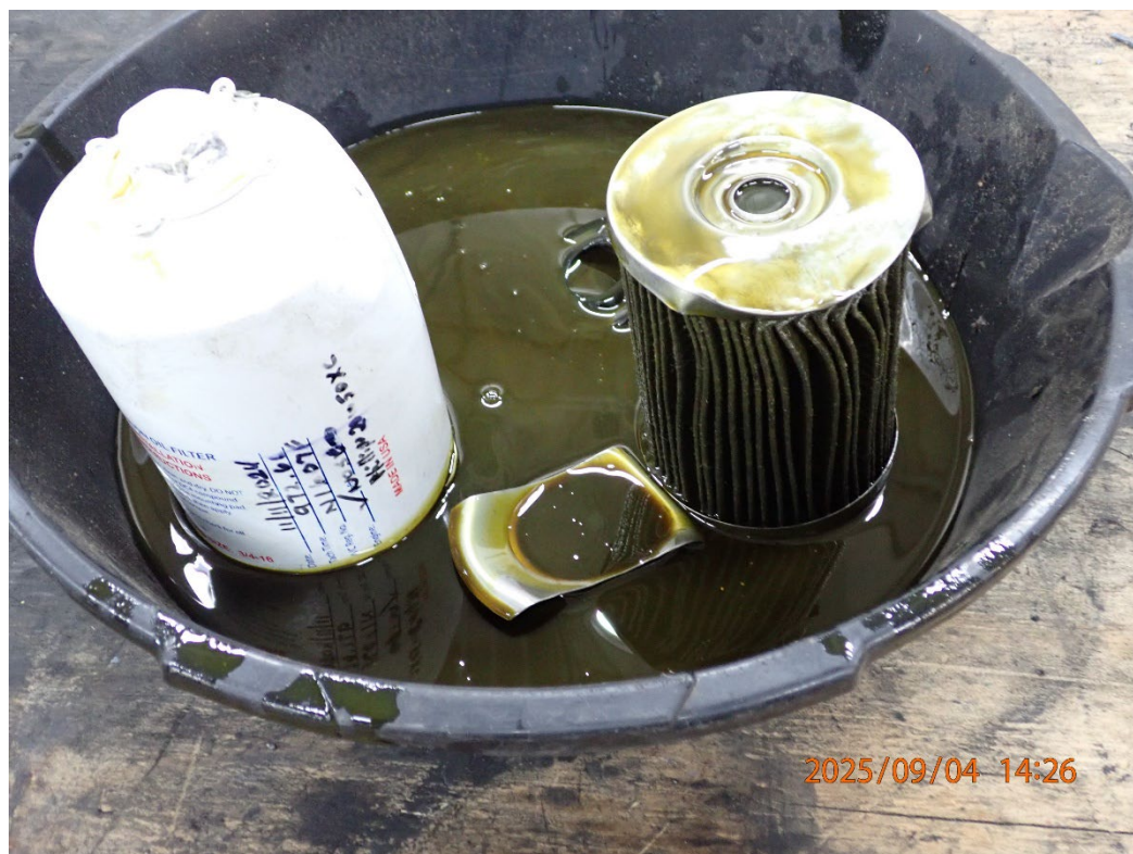
Photo 27: View of the cut open oil filter.
