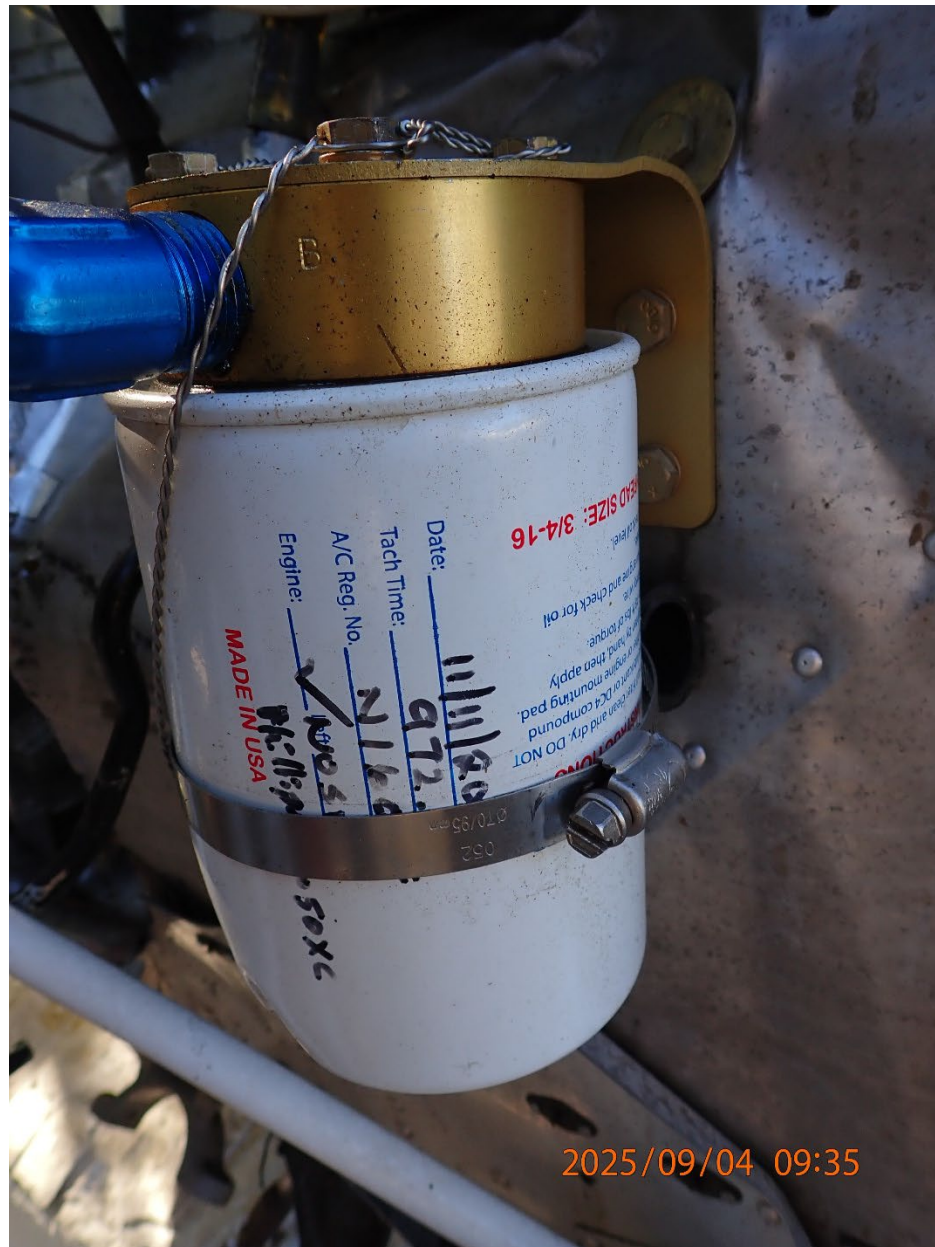
Photo 26: View of the oil filter attached to the oil filter adapter on the firewall.
