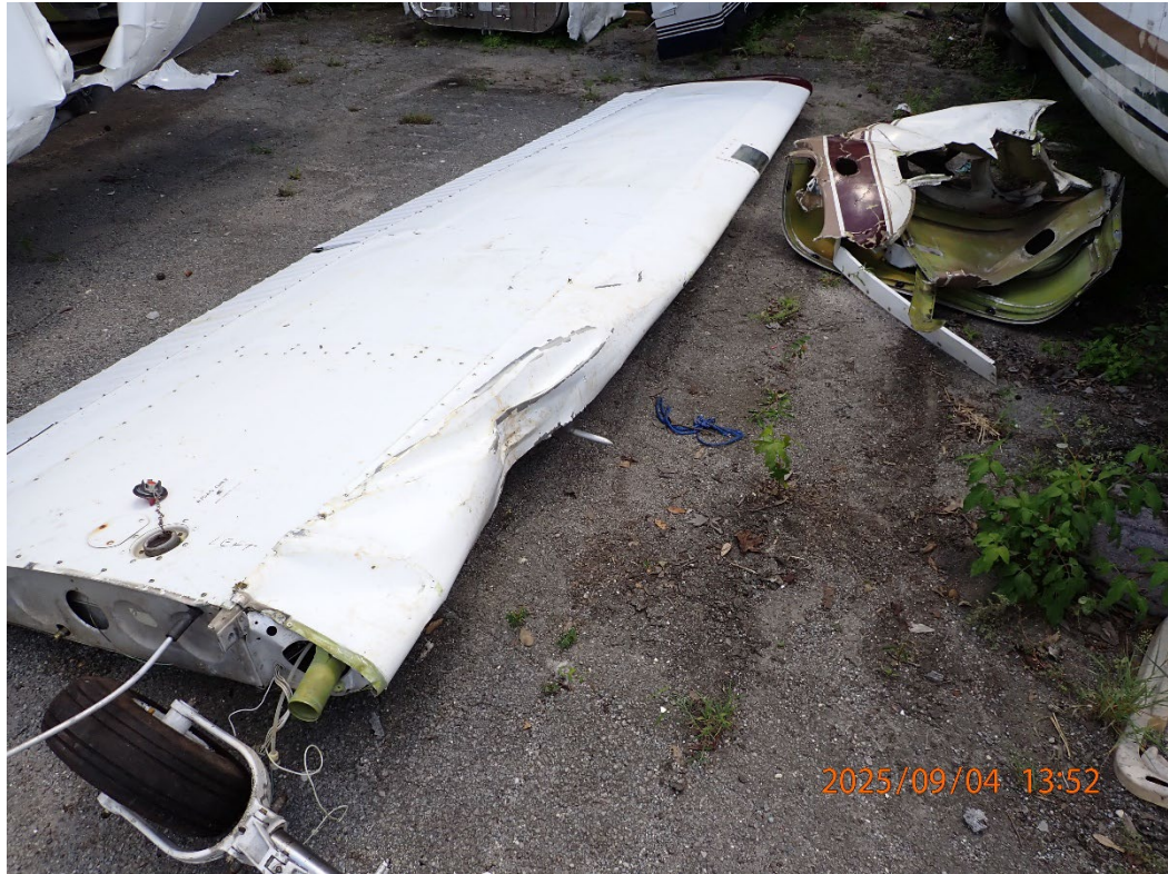
Photo 9: View of damage to the leading edge of the left wing.
