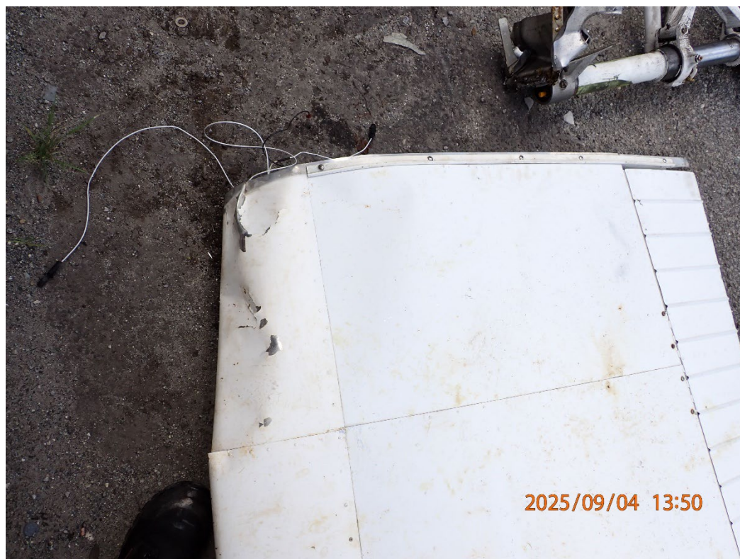
Photo 7: View of damage to the right wingtip.
