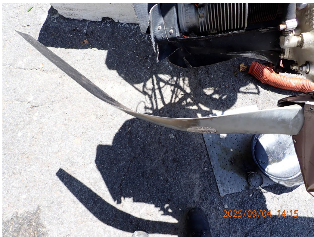
Photo 29: View of the damaged propeller blade.
