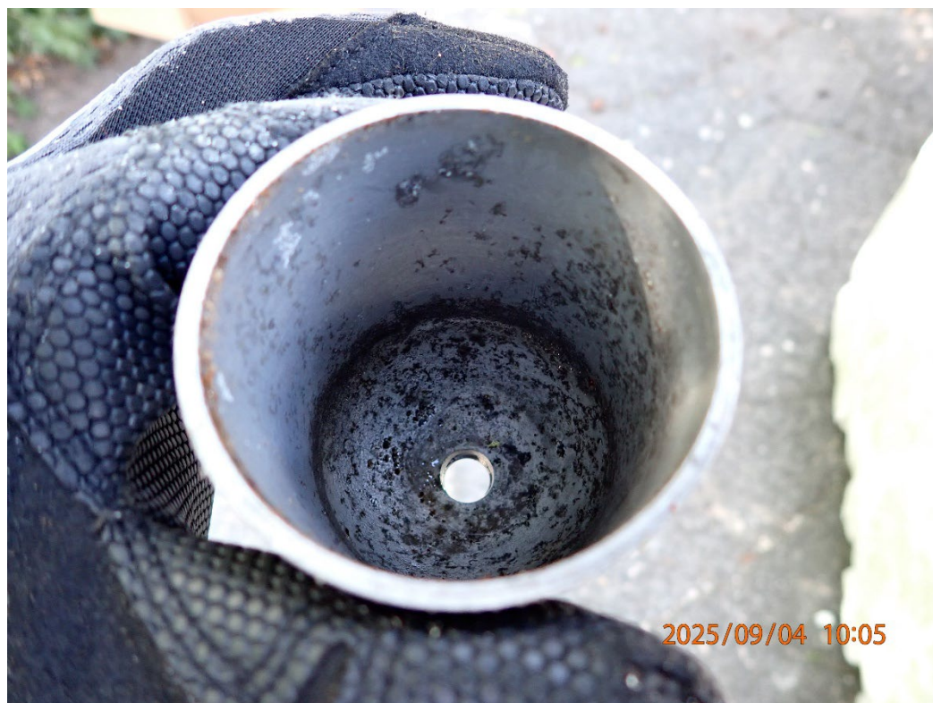
Photo 14: View of the fuel strainer bowl.
