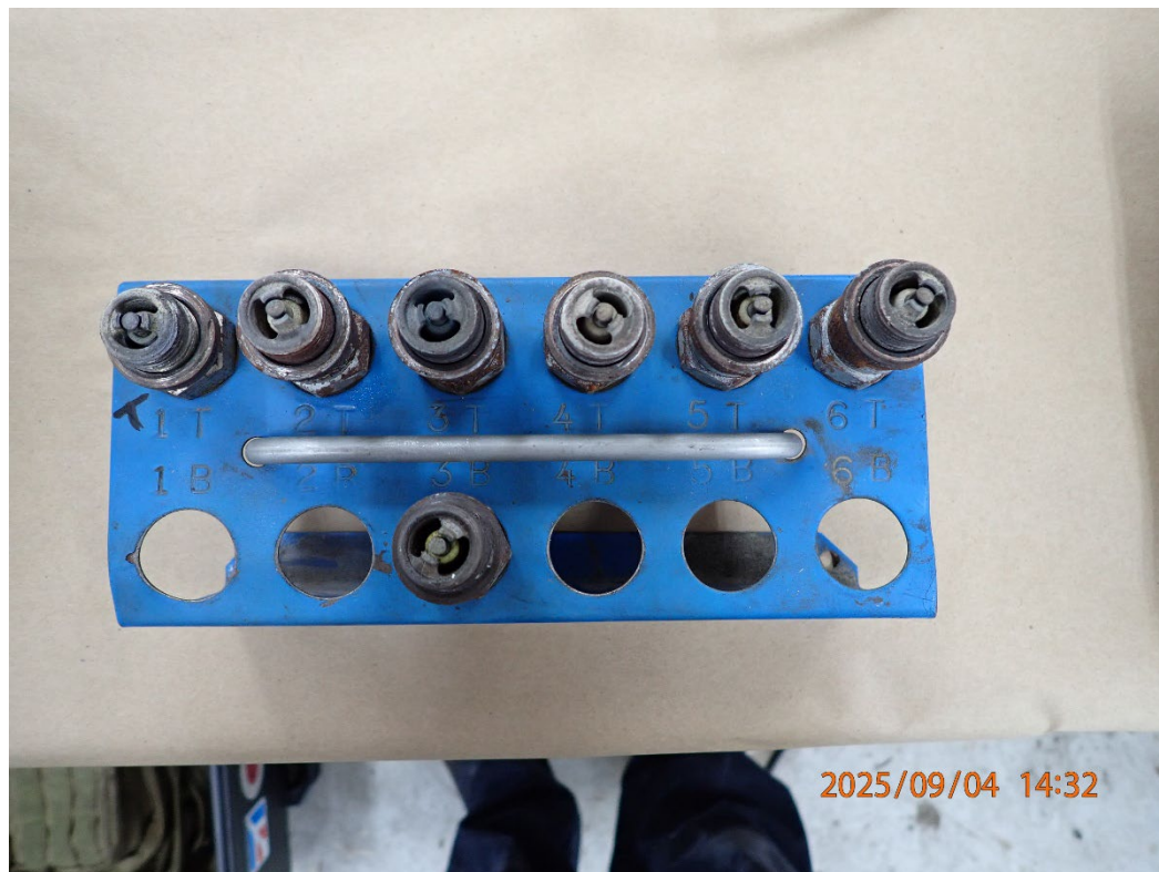
Photo 23: View of the removed sparkplugs.
