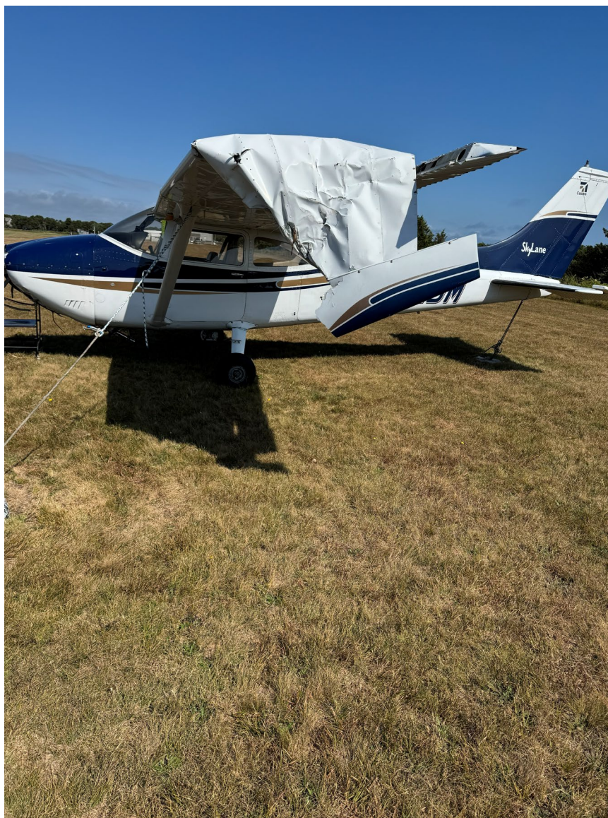
Photograph 3 - Damage to the left wing (Source: FAA)
