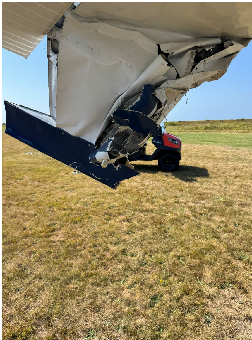
Photograph 4 - Damage to the left wing (Source: FAA)
