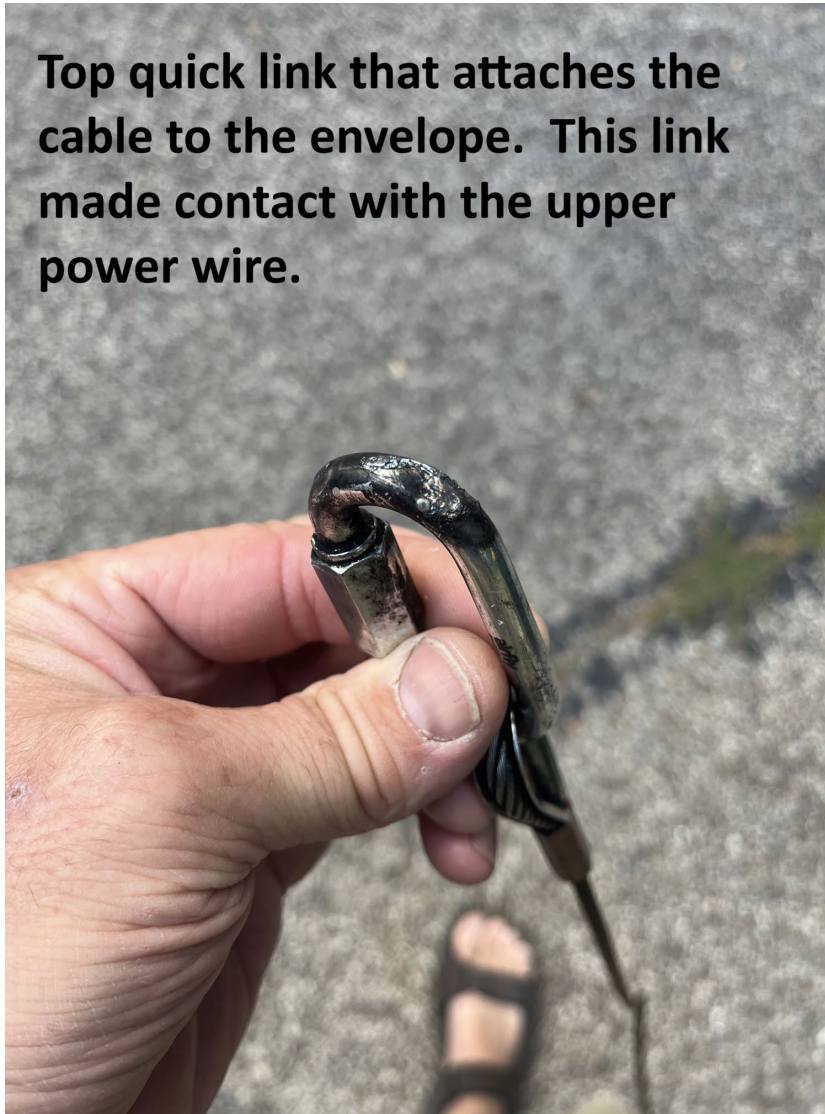
Photograph 1 - Arc on quick link (Courtesy of Owner)
