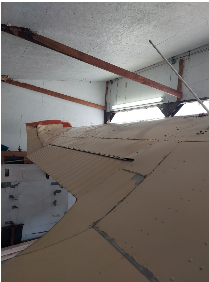
Photograph 1 - Deformation noted to left wing (Courtesy of FAA)
