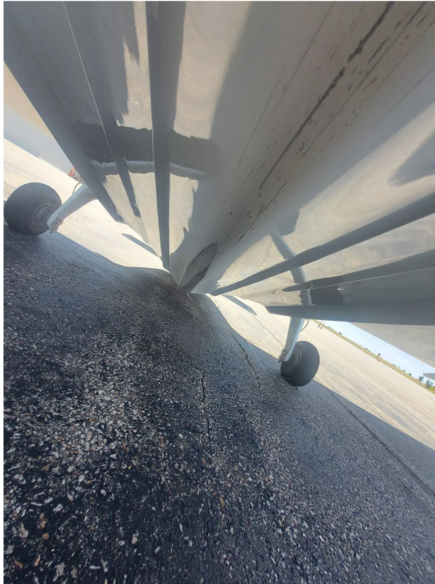
Photograph 2 - Damage to Composite Hull (Courtesy of FAA)
