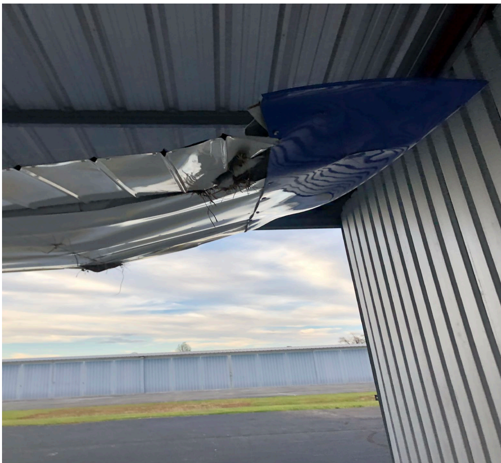
Photograph 2 - View of underside of right wing bent tip. (Courtesy of FAA)
