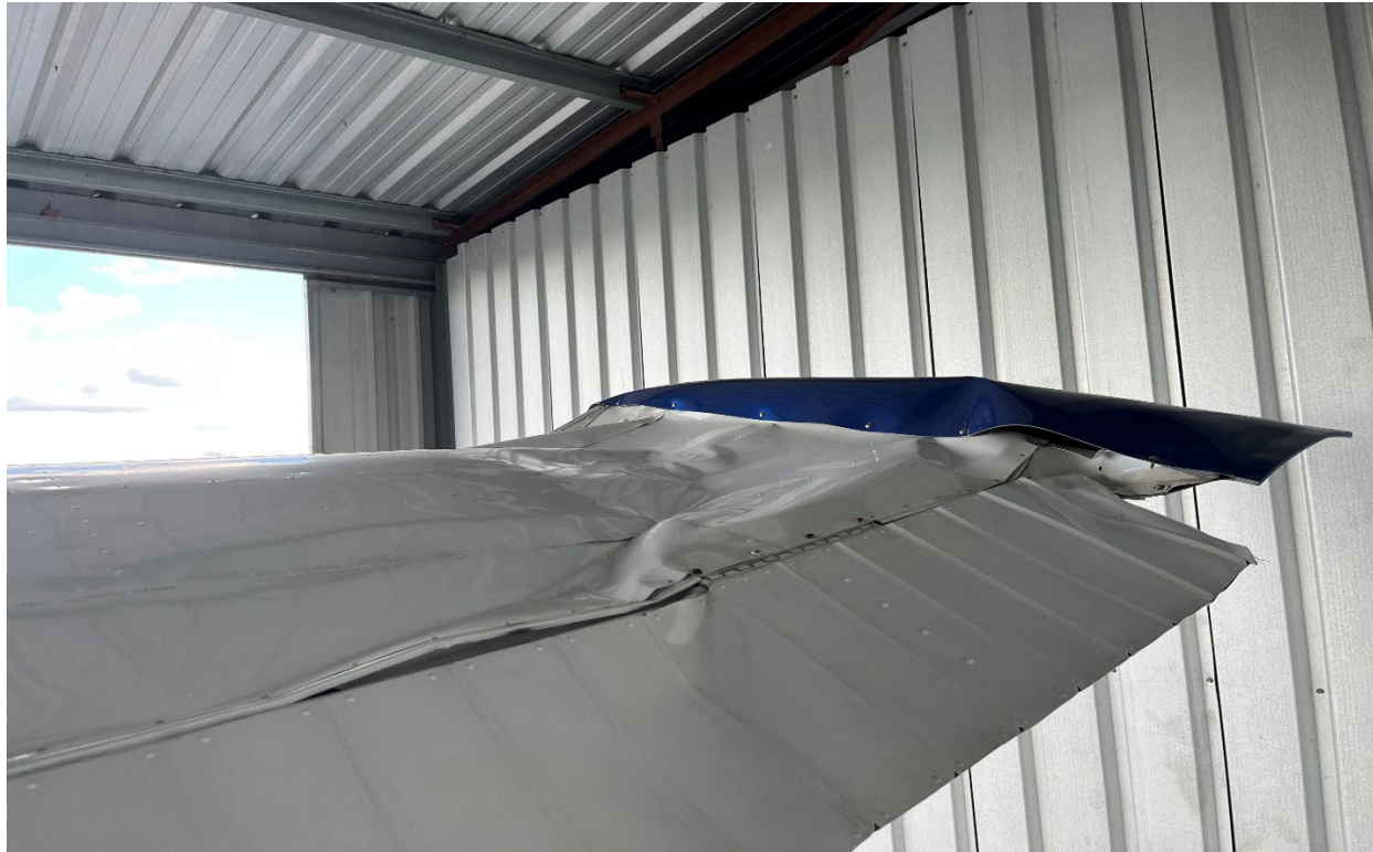
Photograph 3 - View of topside of right wing bent tip. (Courtesy of FAA)
