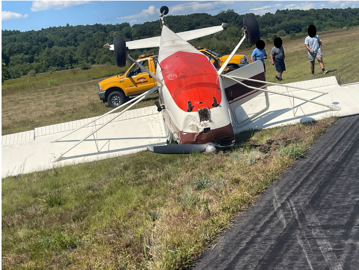
Photograph 2 - Deformation noted to fuselage skin and right-wing lift strut (Courtesy of FAA)
