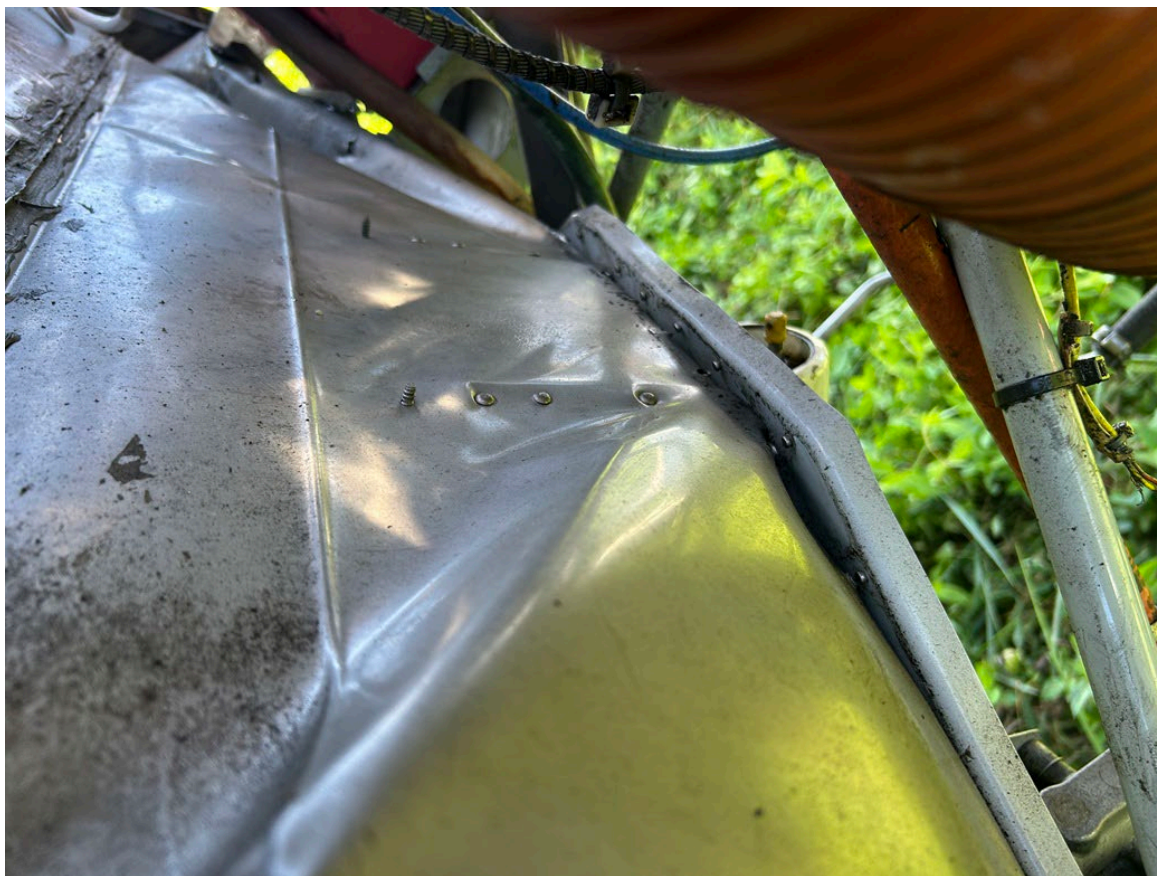
Photograph 3 - Upper Forward Fuselage Damage (Courtesy of FAA)
