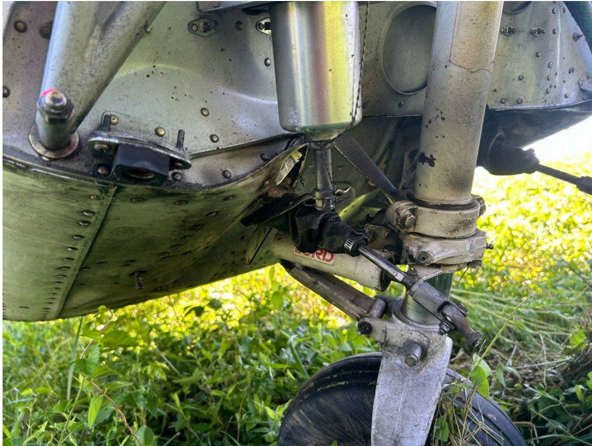
Photograph 2 - Lower Forward Fuselage Damage (Courtesy of FAA)
