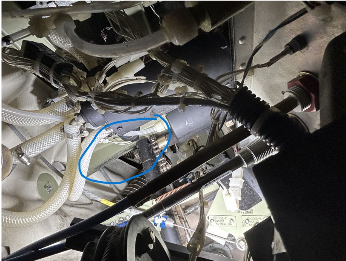
Photograph 5 - Bending of Elevator Control Pivot Point (Courtesy of FAA)
