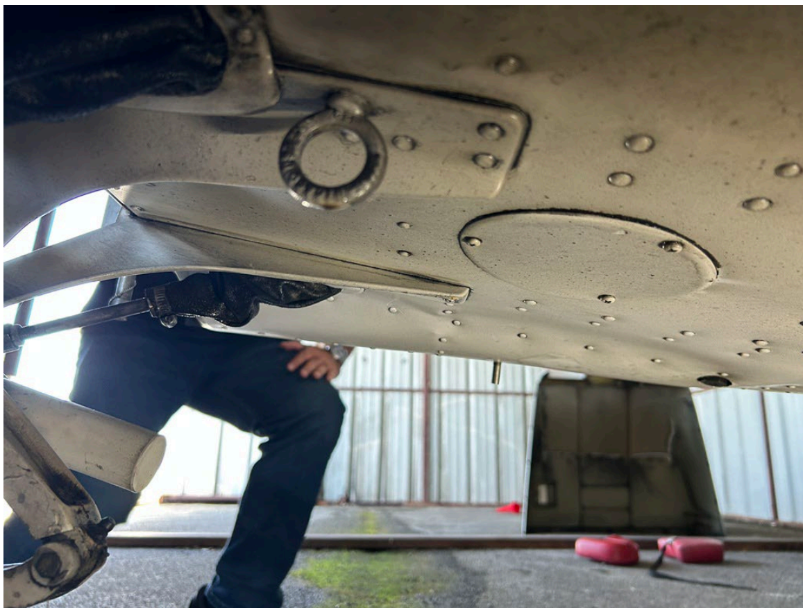
Photograph 4 - Lower Fuselage Impact Damage (Courtesy of FAA)
