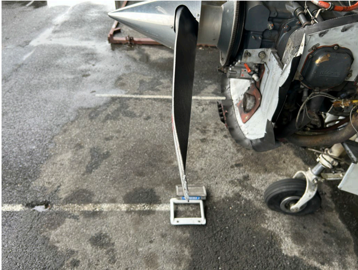
Photograph 1 - Propeller And Nosewheel Tire Damage (Courtesy of FAA)
