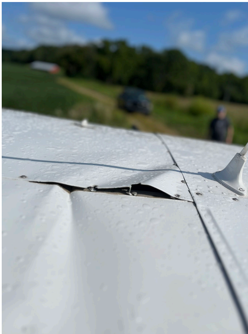
Photograph 2 - Left upper wing root view (Courtesy of FAA)
