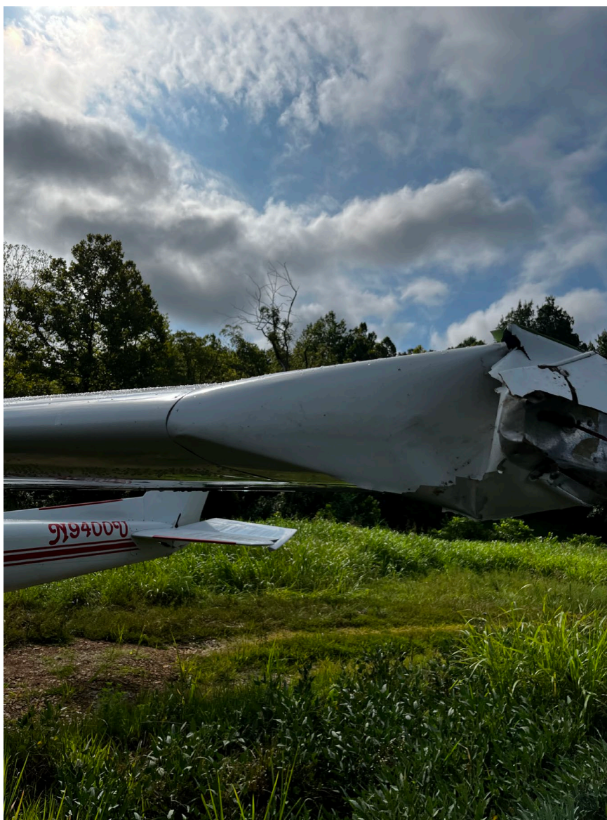
Photograph 3 - left wing tip damage (Courtesy of FAA)
