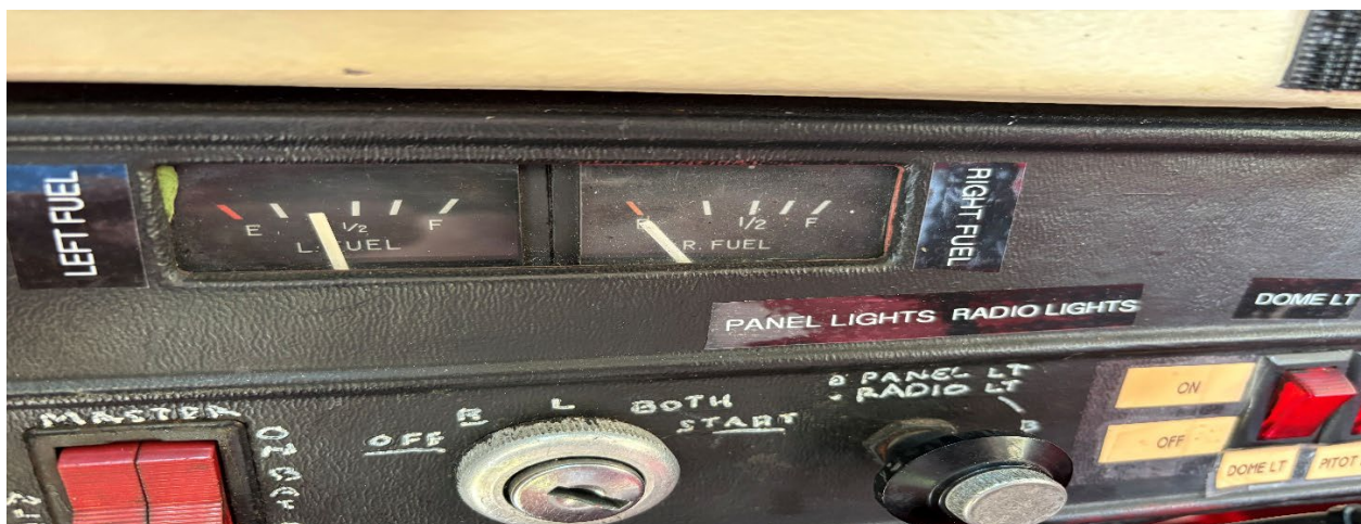
Left fuel tank reading over a \frac{1}{4} tank of fuel, but void of fuel. (FAA Photo)
