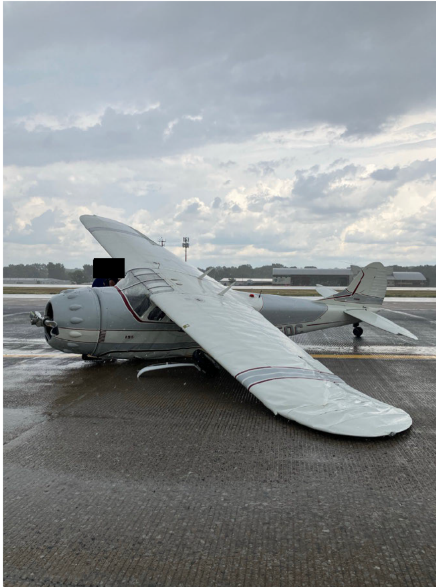
Photograph 2 - Damage to Left Wing, Fuselage, and Landing Gear (Courtesy of FAA)
