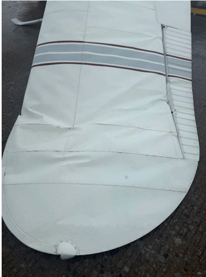
Photograph 3 - Left Wing Damage (Courtesy of FAA)
