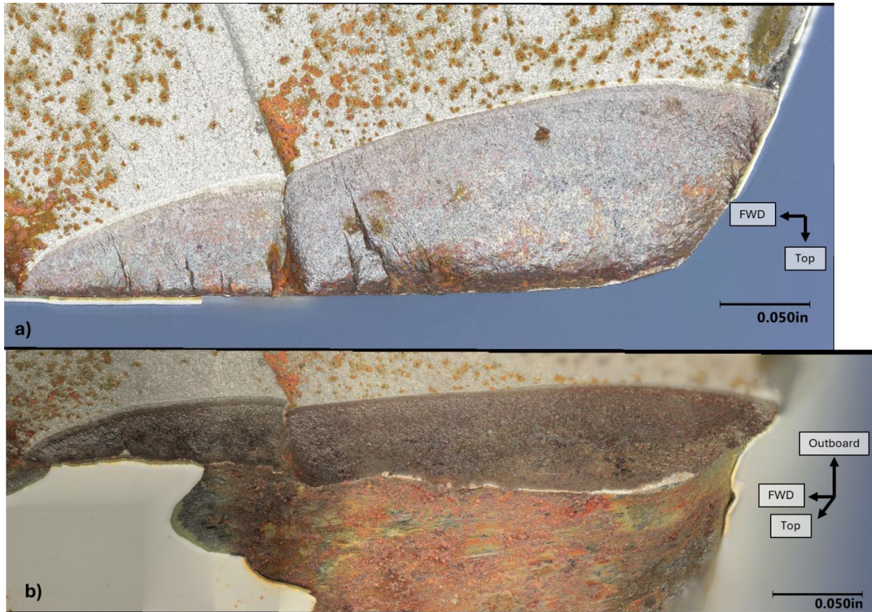
Figure 7. Digital microscopic images of the thumbnail crack a) top down highlighting the region and beachmark at the crack tip, and b) oblique angle to show adjacent component surface.
