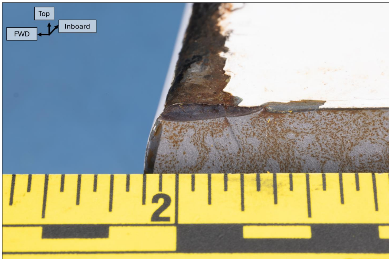
Figure 6. As-received photograph at an oblique angle of the thumbnail crack and wear surface.
