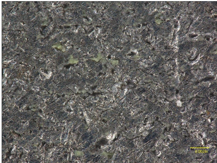
Figure 16. Digital microscopic image of an area away from the crack and worn region, exhibiting pit-like texturing. Remnant primer material can be observed in the cavities of the surface, suggesting the pits were present at time of primer application.
