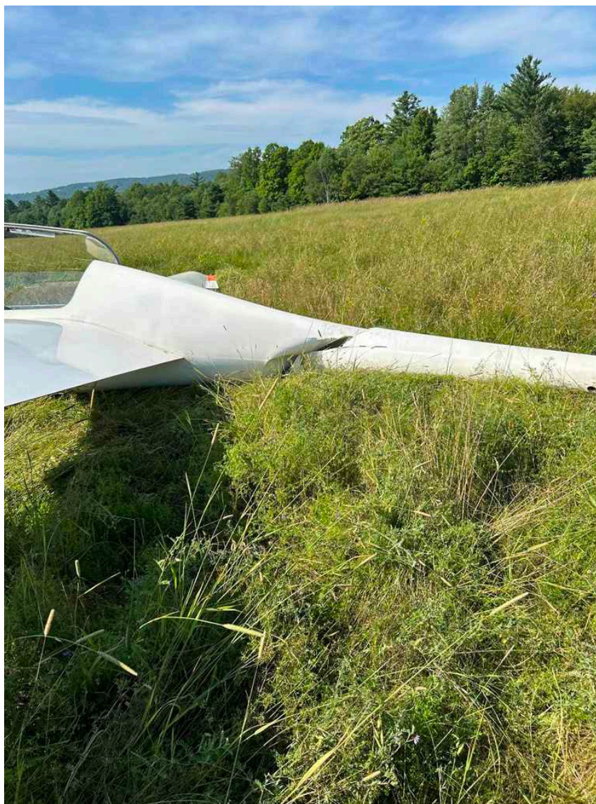
Photograph 1 -Glider in Field with Broken Tail Boom (Courtesy of FAA)
