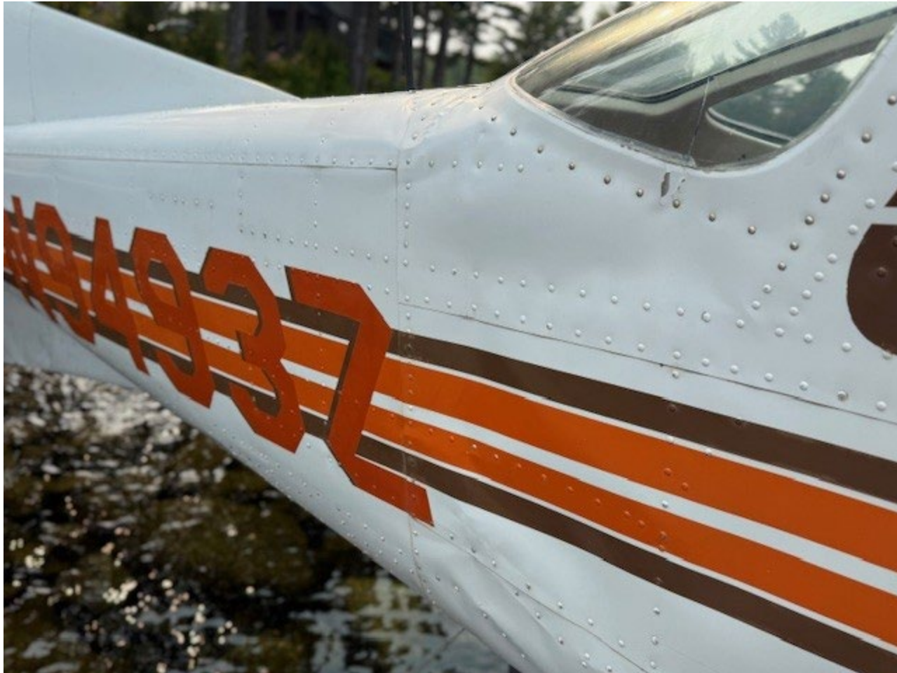
Photograph 1 - View of damage to the fuselage. (Courtesy of Pilot)
