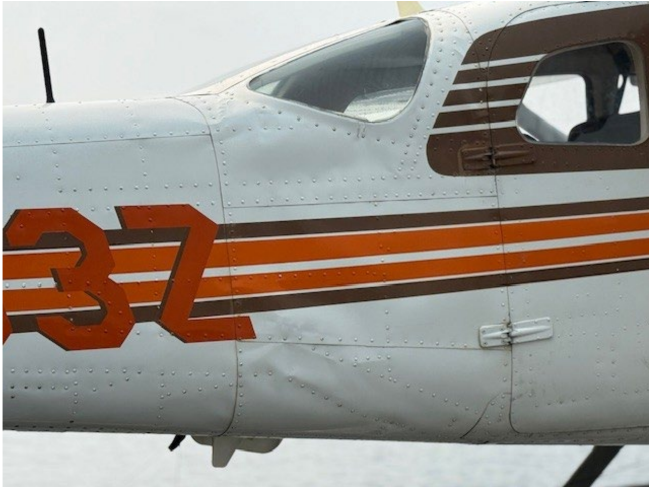
Photograph 2 - View of fuselage damage. (Courtesy of Pilot)
