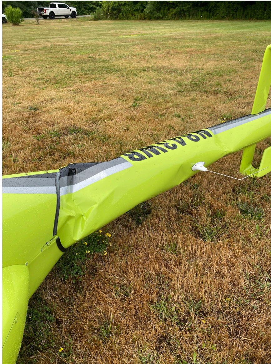
Photograph 3 - View Showing Damage to the Tailboom (Courtesy of FAA)
