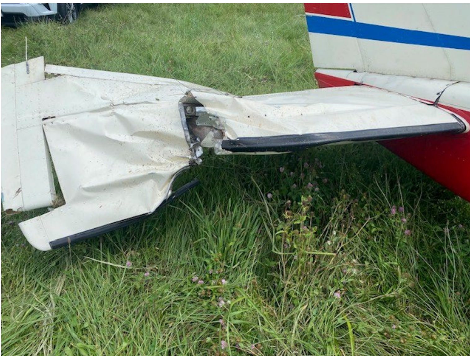
Photograph 1 - right horizontal stabilizer (Courtesy of FAA)
