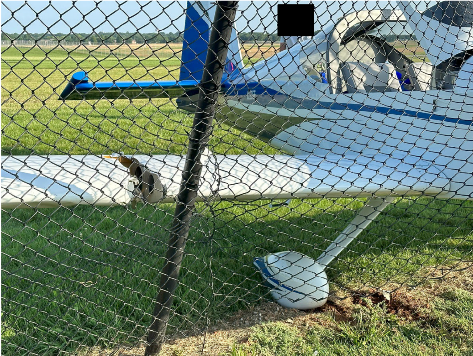
Photograph 3 – Damage to the right wing (Source: Pilot)
