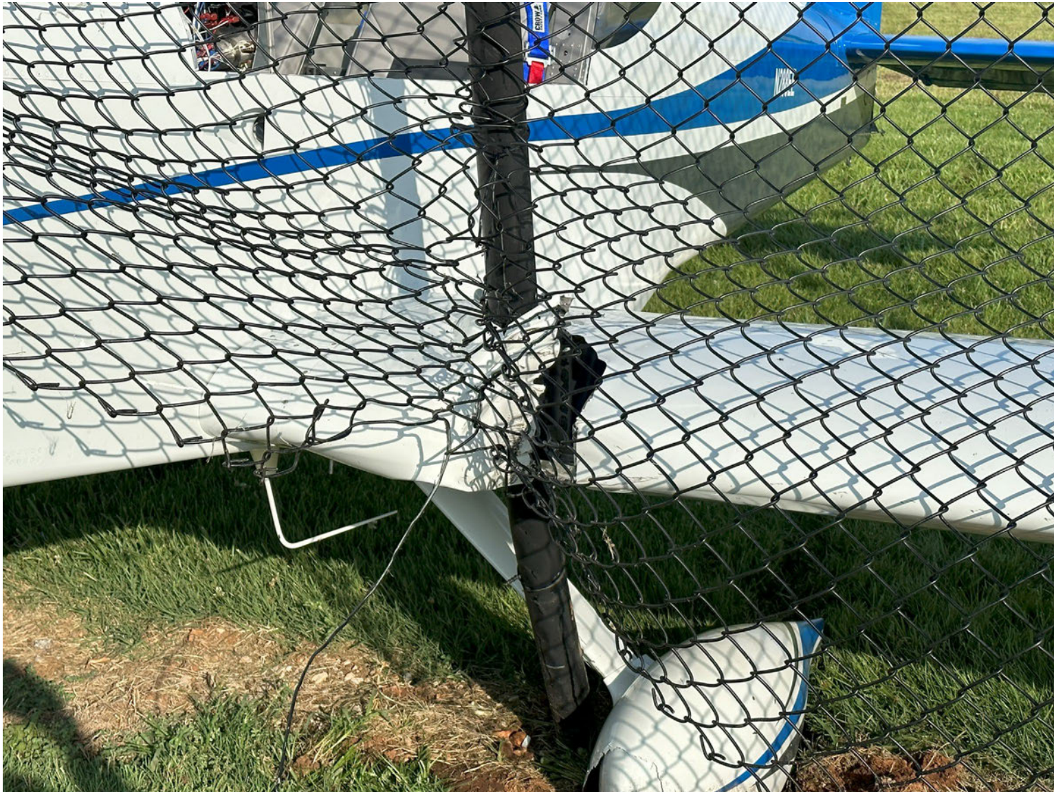
Photograph 4 – Damage to the left wing (Source: Pilot)
