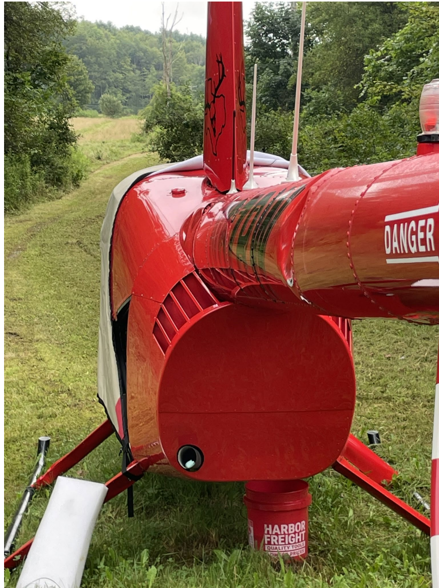
Photograph 1 - View of damage to the tail boom. (Courtesy of FAA)
