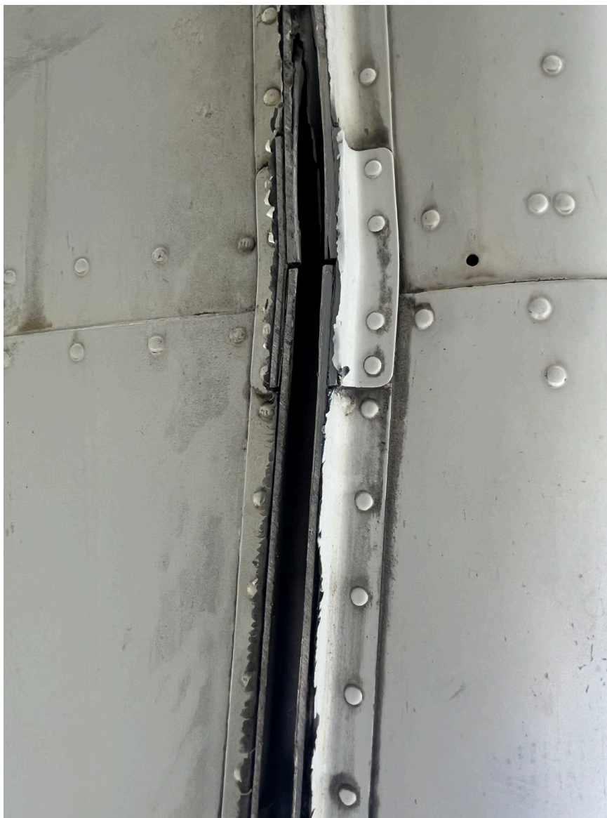
Photograph 6 - Close-Up View Showing Damage to External Longeron (Courtesy of FAA)
