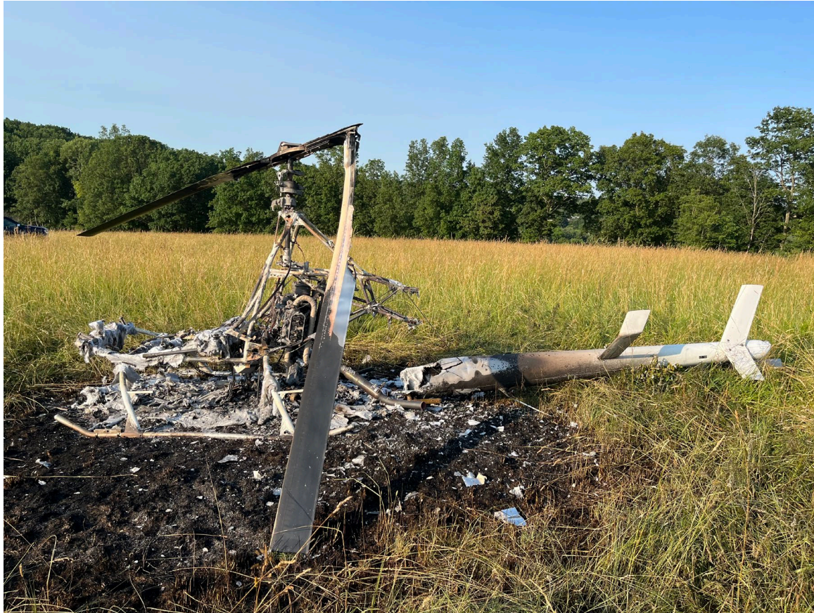
Photograph 4 - Left-side view of post-crash fire damaged helicopter. (Courtesy of FAA)
