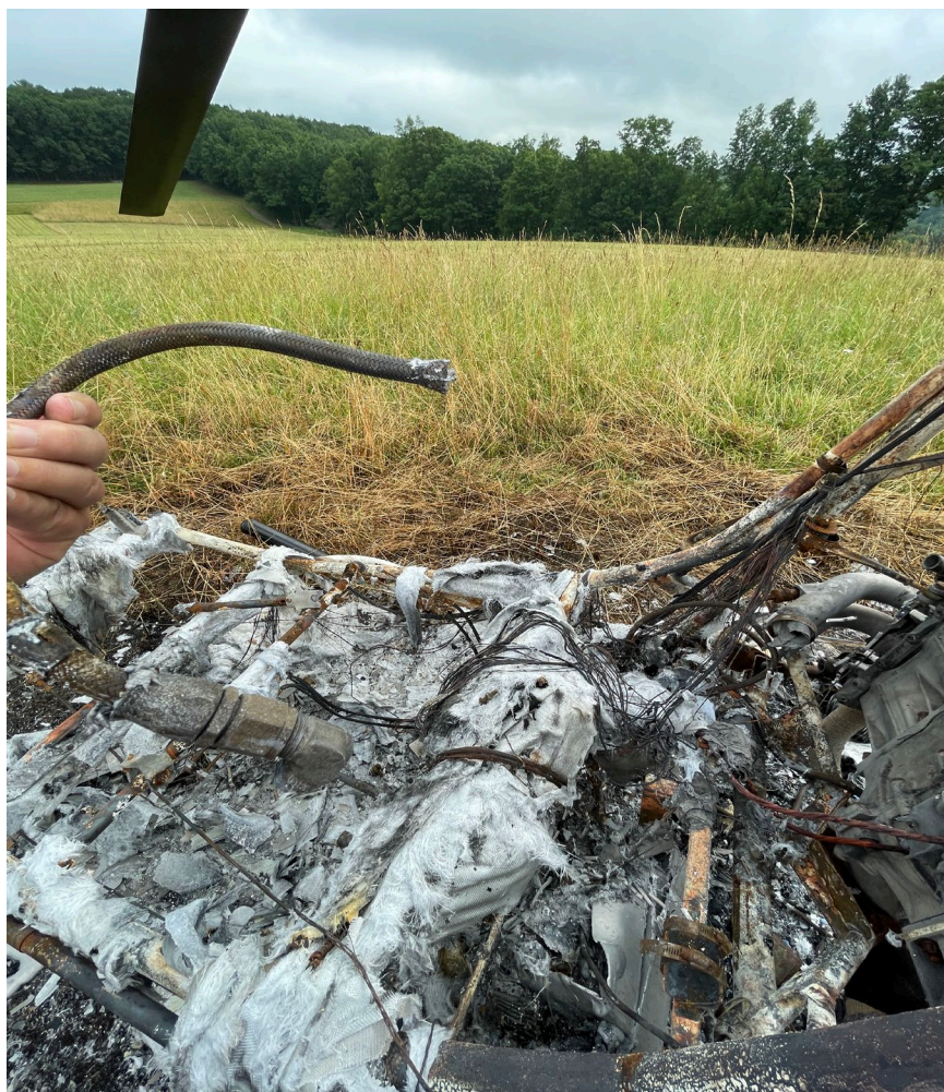
Photograph 6 - View of fire damaged fuel lines. (Courtesy of FAA)
