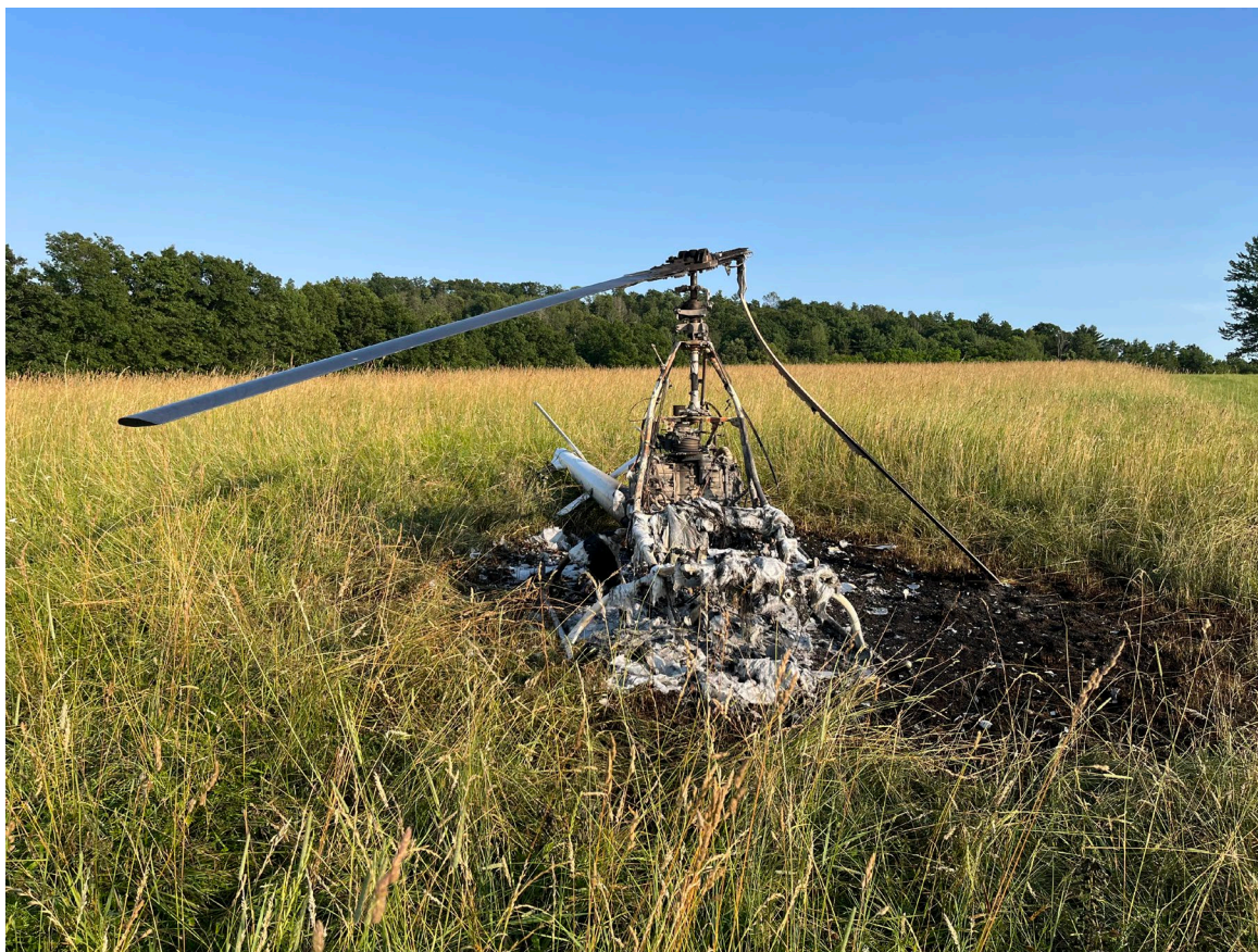
Photograph 1 - Forward view of upright post-crash fire damaged helicopter. (Courtesy of FAA)
