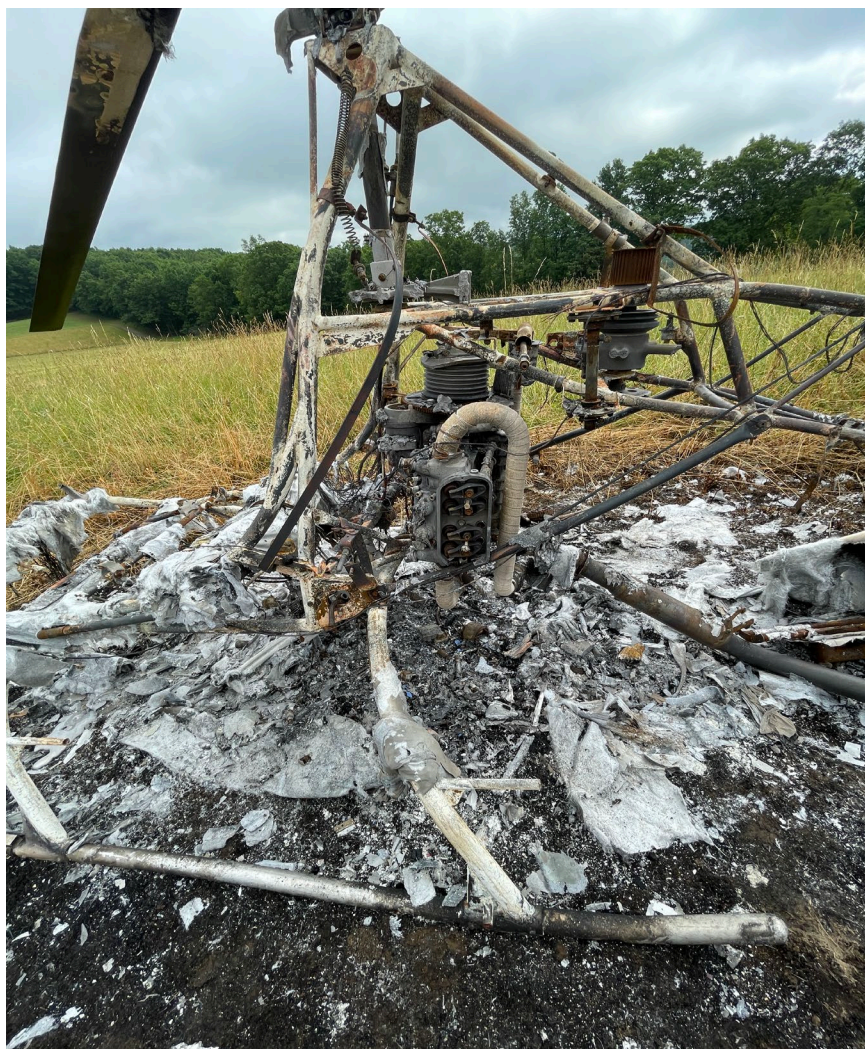
Photograph 5 - View of post-crash fire damaged engine. (Courtesy of FAA)
