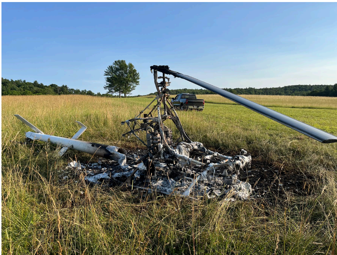
Photograph 2 - Right-side view of upright post-crash fire damaged helicopter. (Courtesy of FAA)
