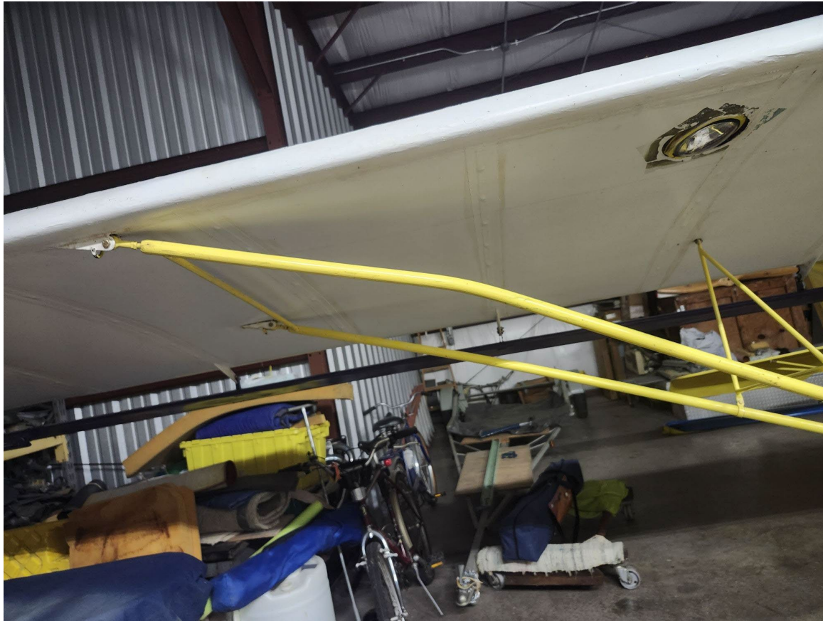
Photograph 2 - Right wing strut accident damage (Courtesy of Pilot)
