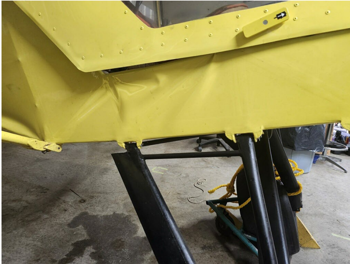
Photograph 4 - Right side fuselage buckling (Courtesy of Pilot)
