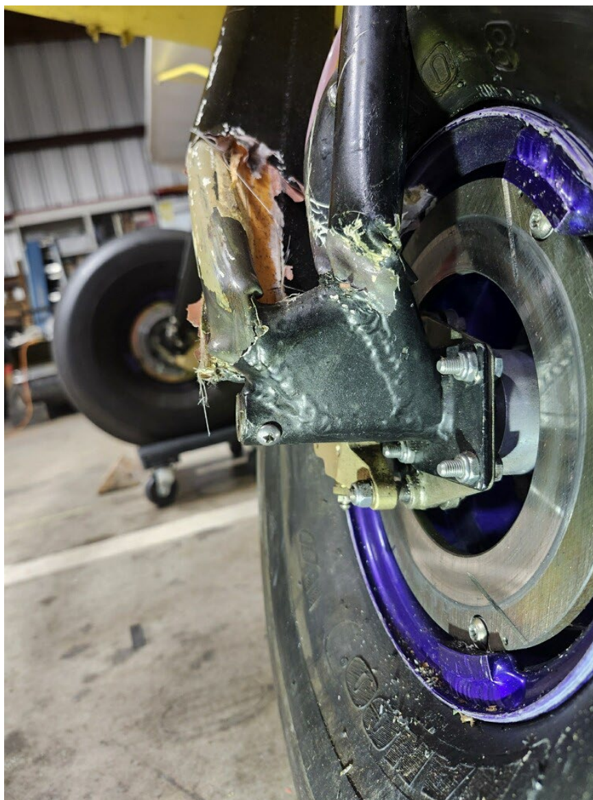
Photograph 5 - Left main landing gear damage (Courtesy of Pilot)
