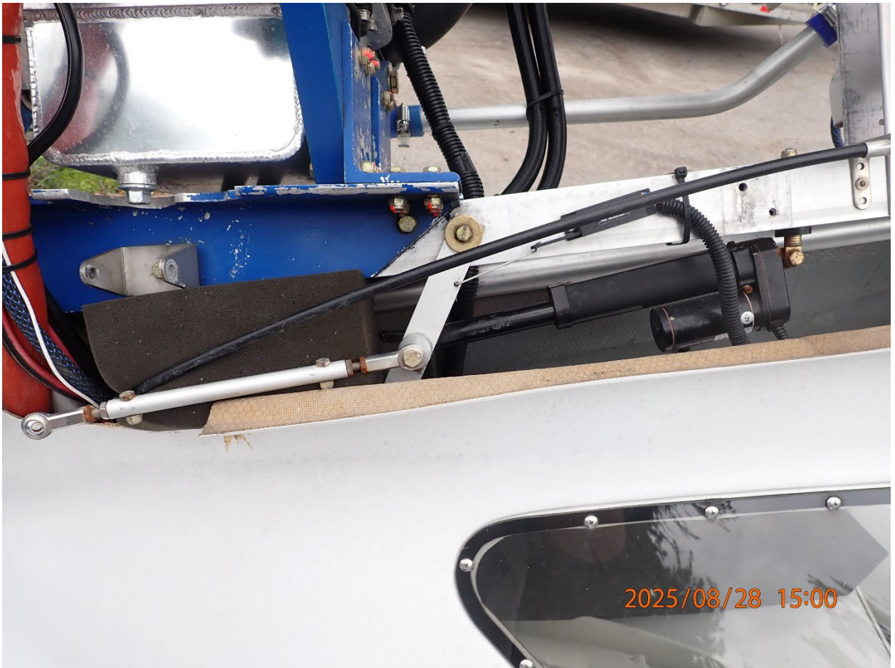
Figure 1: View of the flap actuator and motor as found.
