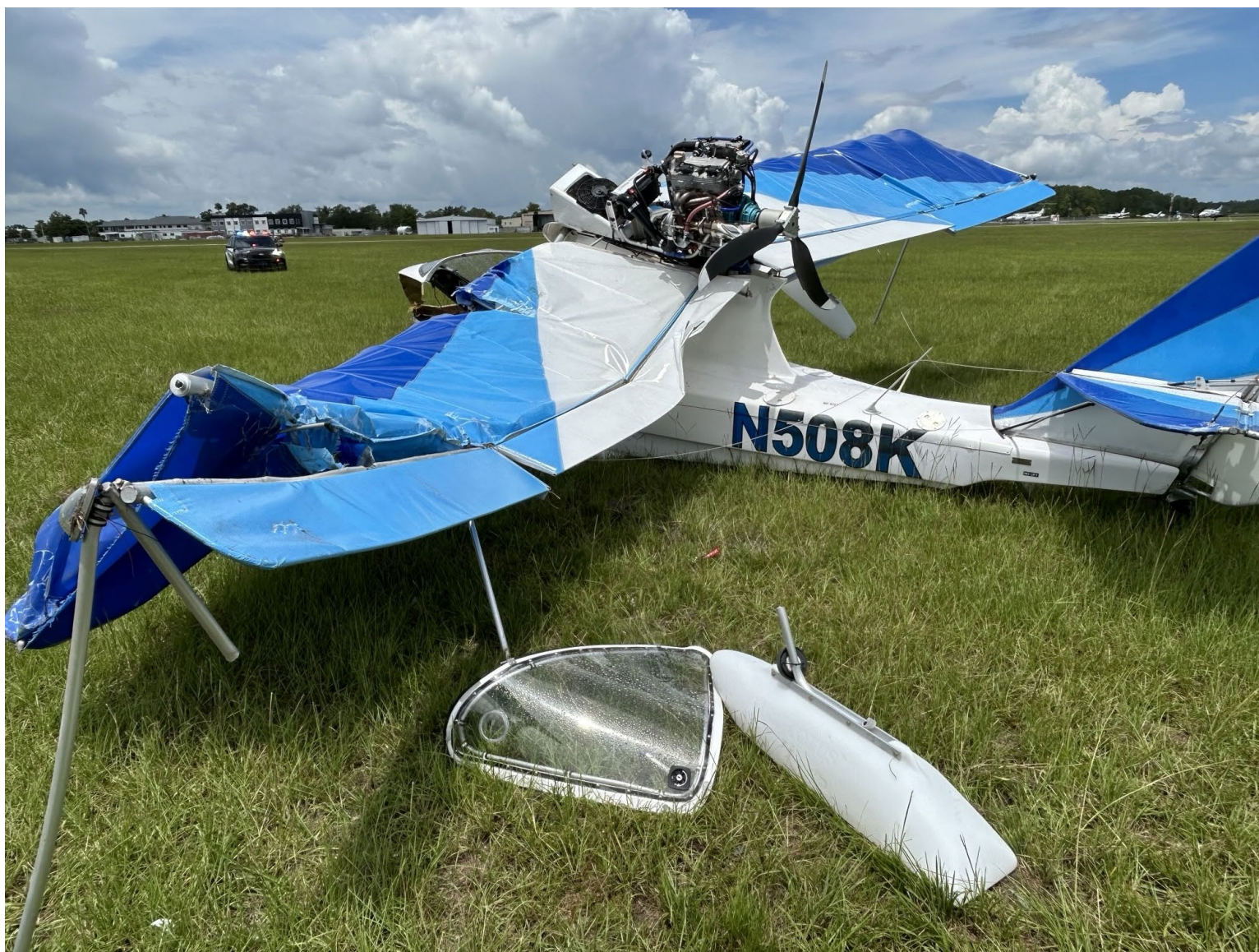
Photograph 2 - View of damage to the airplane. (Courtesy of Airport Manager)
