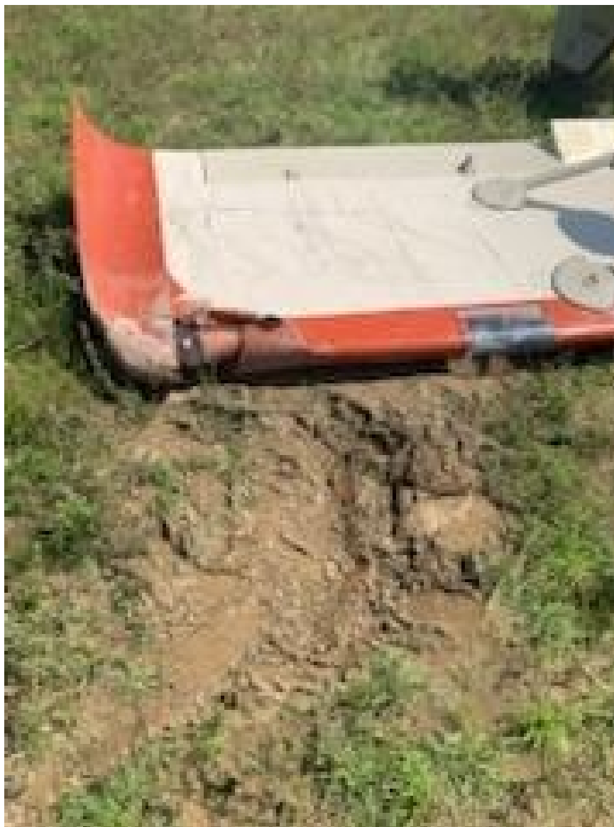
Photograph 3 - Left wing damage. (Courtesy of Pilot)
