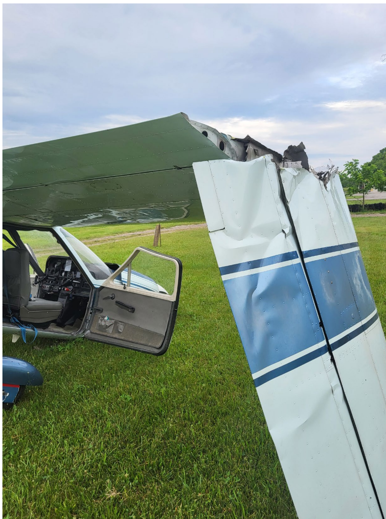
Photograph 1 - View of right wing damage. (Courtesy of Pilot)
