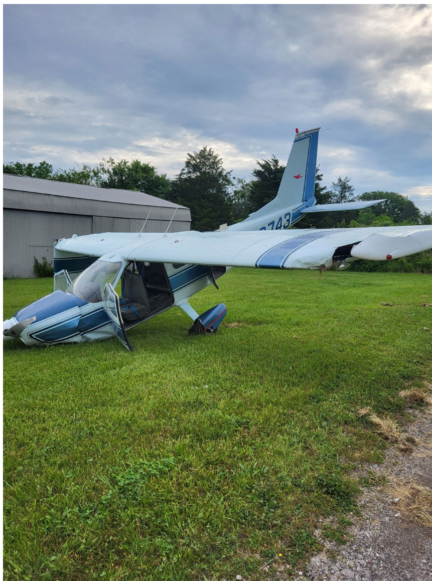
Photograph 3 - View of left wing, right wing, and fuselage damage. (Courtesy of Pilot)
