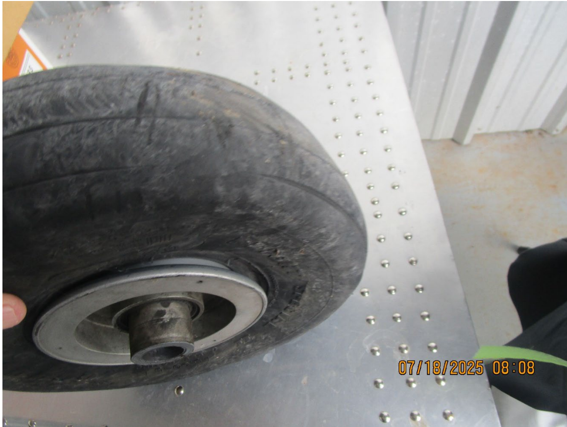
Photograph 7 - Nose wheel showing no rim damage (Courtesy of FAA)
