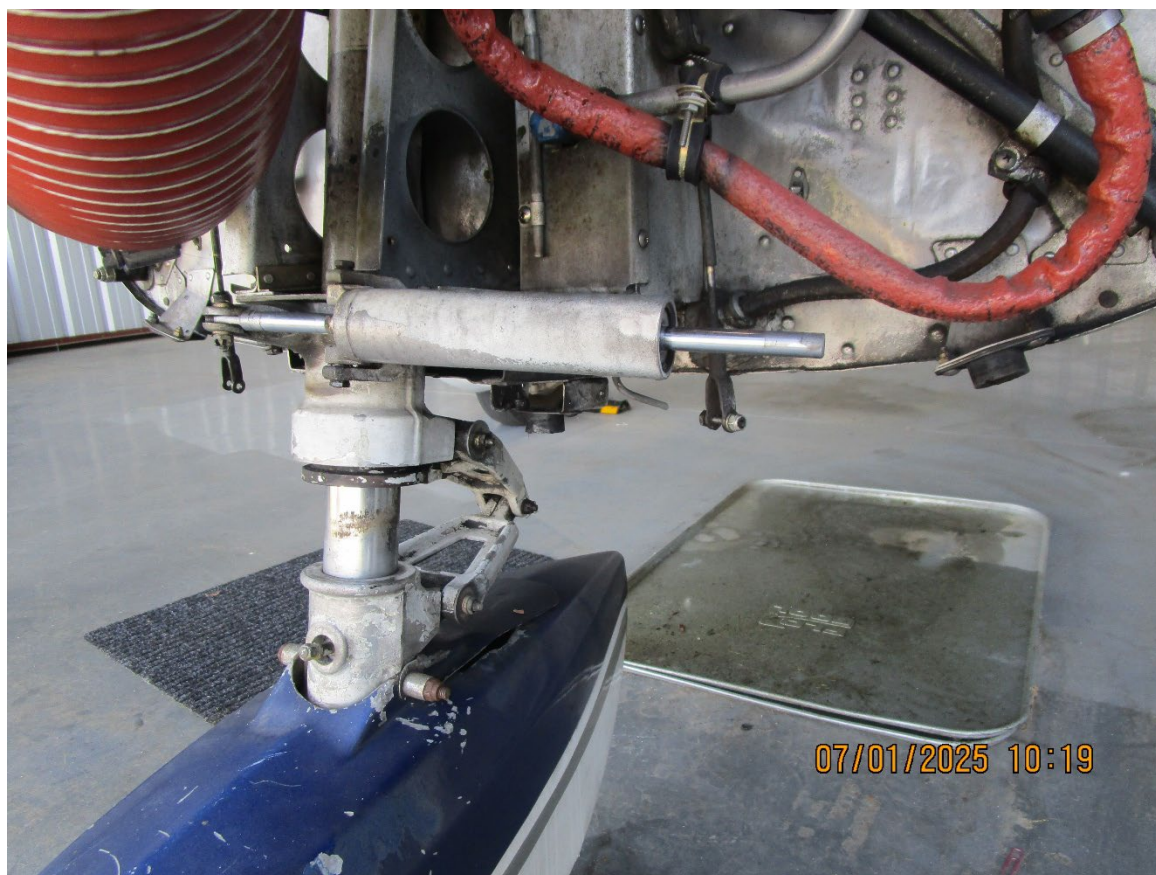
Photograph 6 - Damage to lower firewall and supporting structure (Courtesy of FAA)
