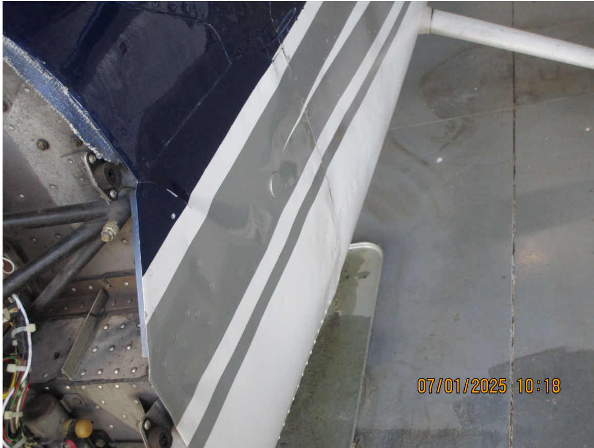
Photograph 5 - Close up of damage to left side of fuselage (Courtesy of FAA)
