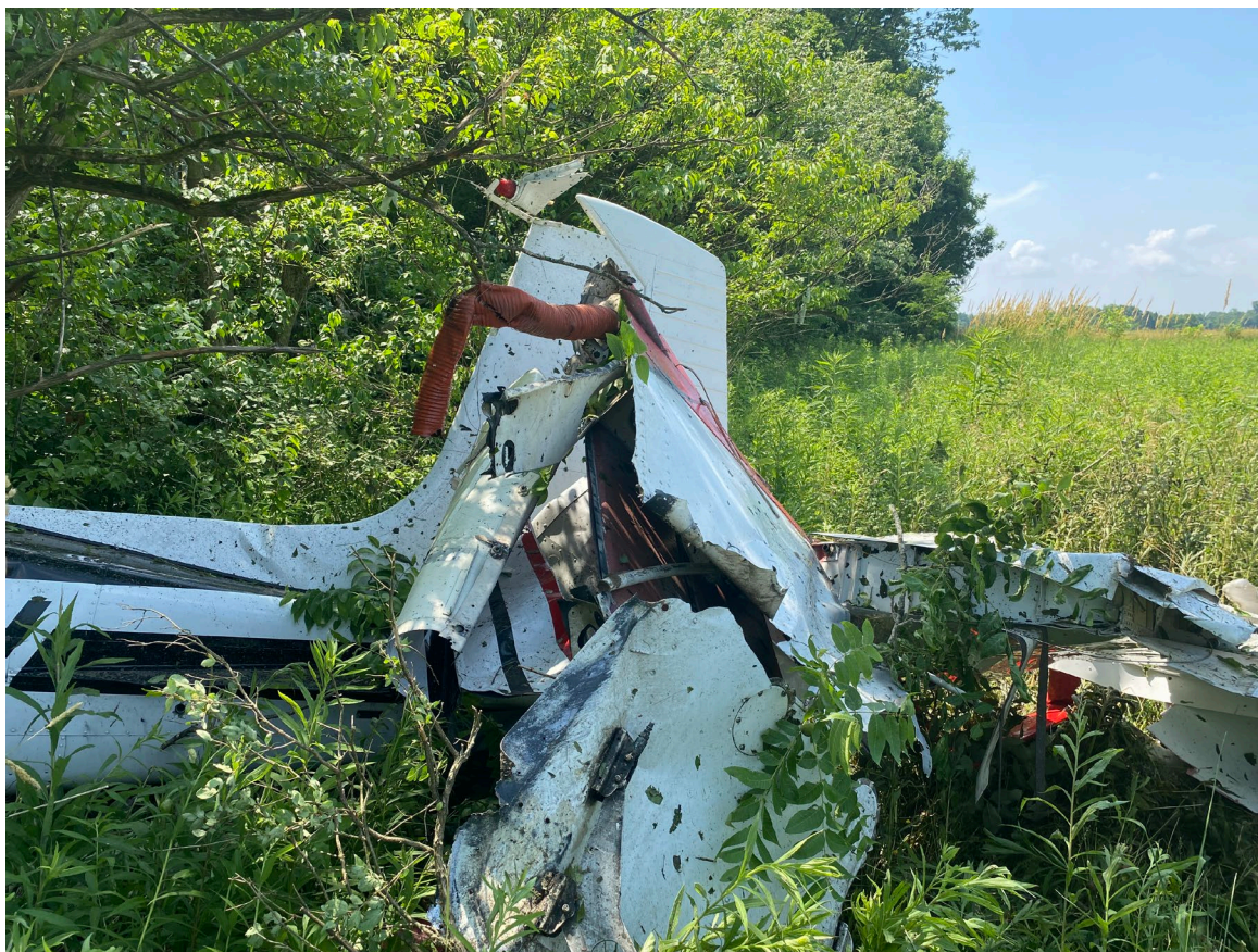
Photograph 2 - Impact separated left wing (Courtesy of FAA)
