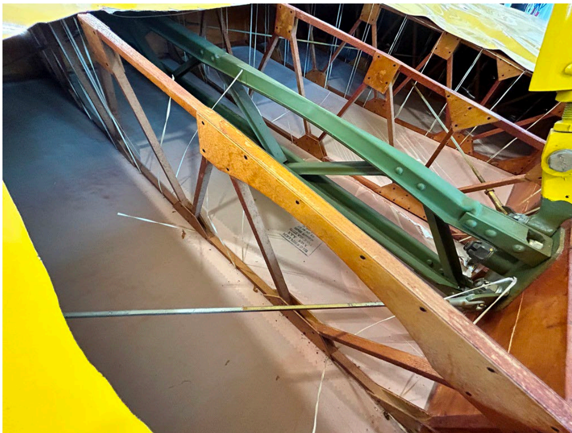
Photograph 3 - Damaged Lower Right Wing Spar (Courtesy of FAA)
