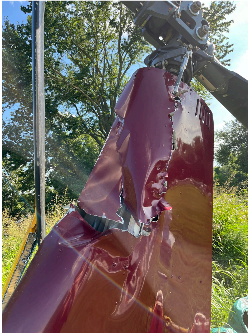
Photograph 6 - Rotor mast damage (Courtesy of NTSB)
