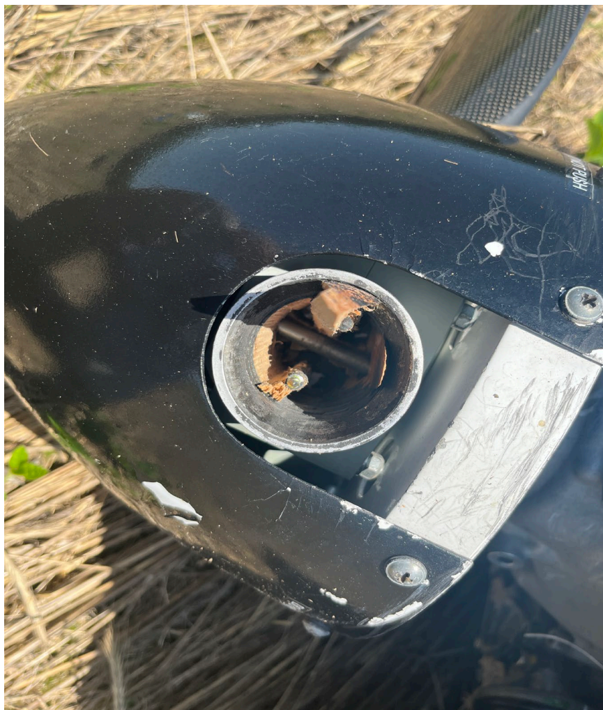
Photograph 3 - View of missing #1 propeller out of propeller hub. (Courtesy of FAA)
