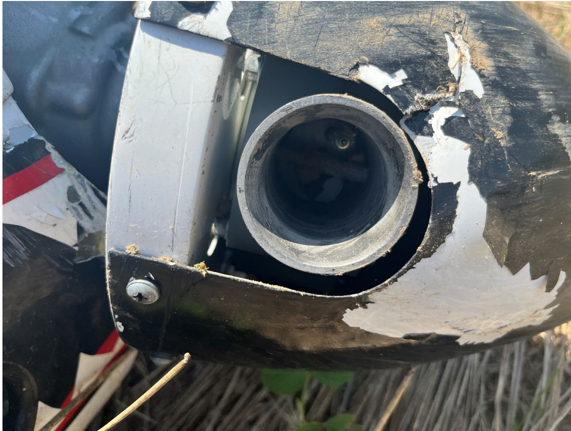
Photograph 4 - View of #2 propeller missing from propeller hub. (Courtesy of FAA)
