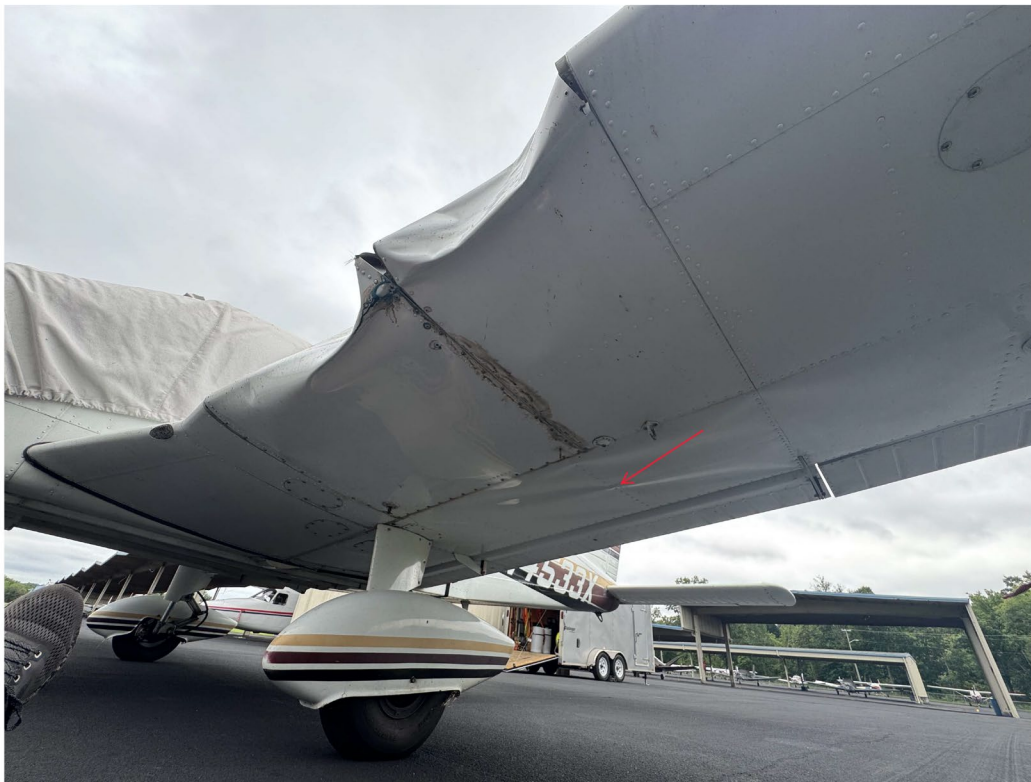
Photograph 2 - FAA Digital Photograph. View of the Bottom of a Portion of the Left Wing. Arrow Points to Buckling of the Lower Wing Skin Aft of the Main Spar
