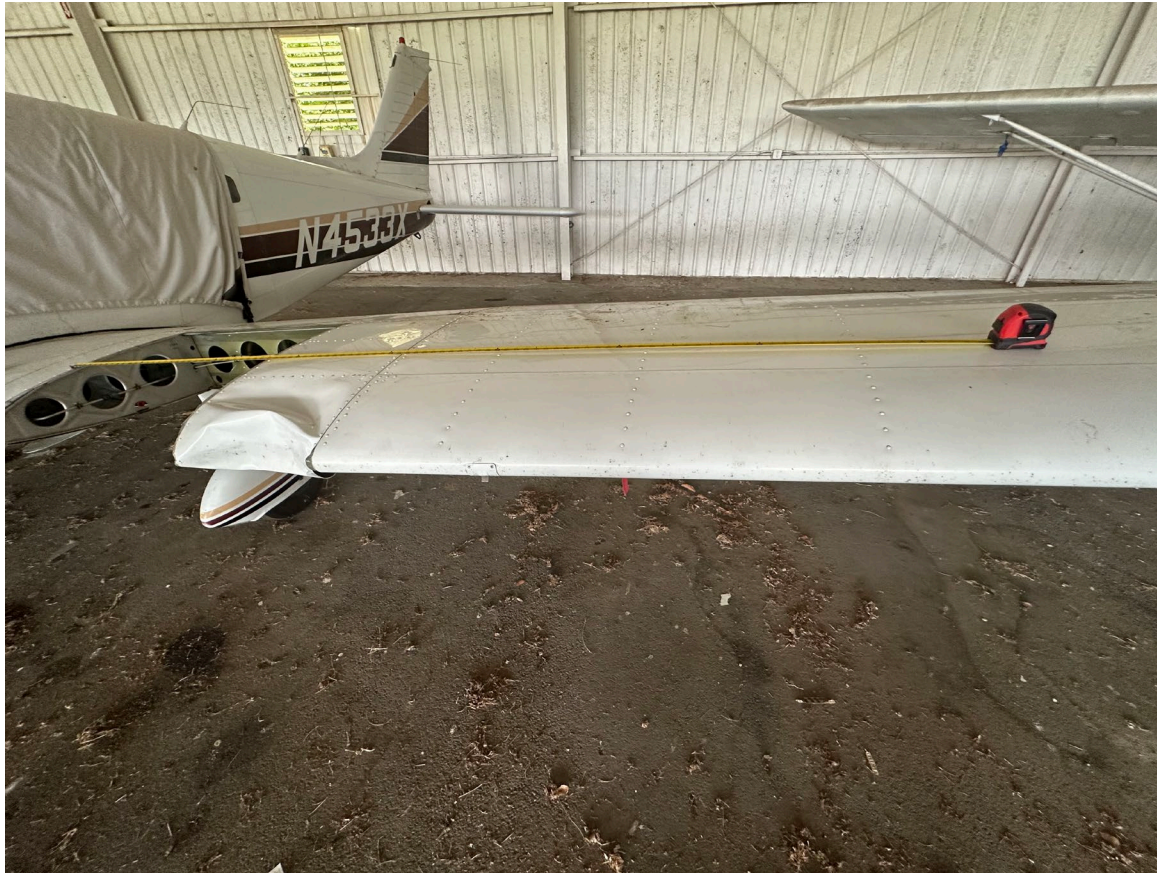
Photograph 3 - FAA Digital Photograph. View Showing the Approximate 48 Inches of Span Damage to the Leading Edge
