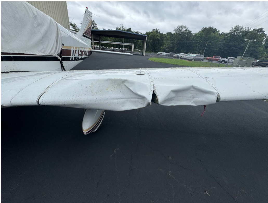
Photograph 1 - FAA Digital Photograph. Frontal View of a Portion of the Left Wing Showing the Leading Edge Impact Damage
