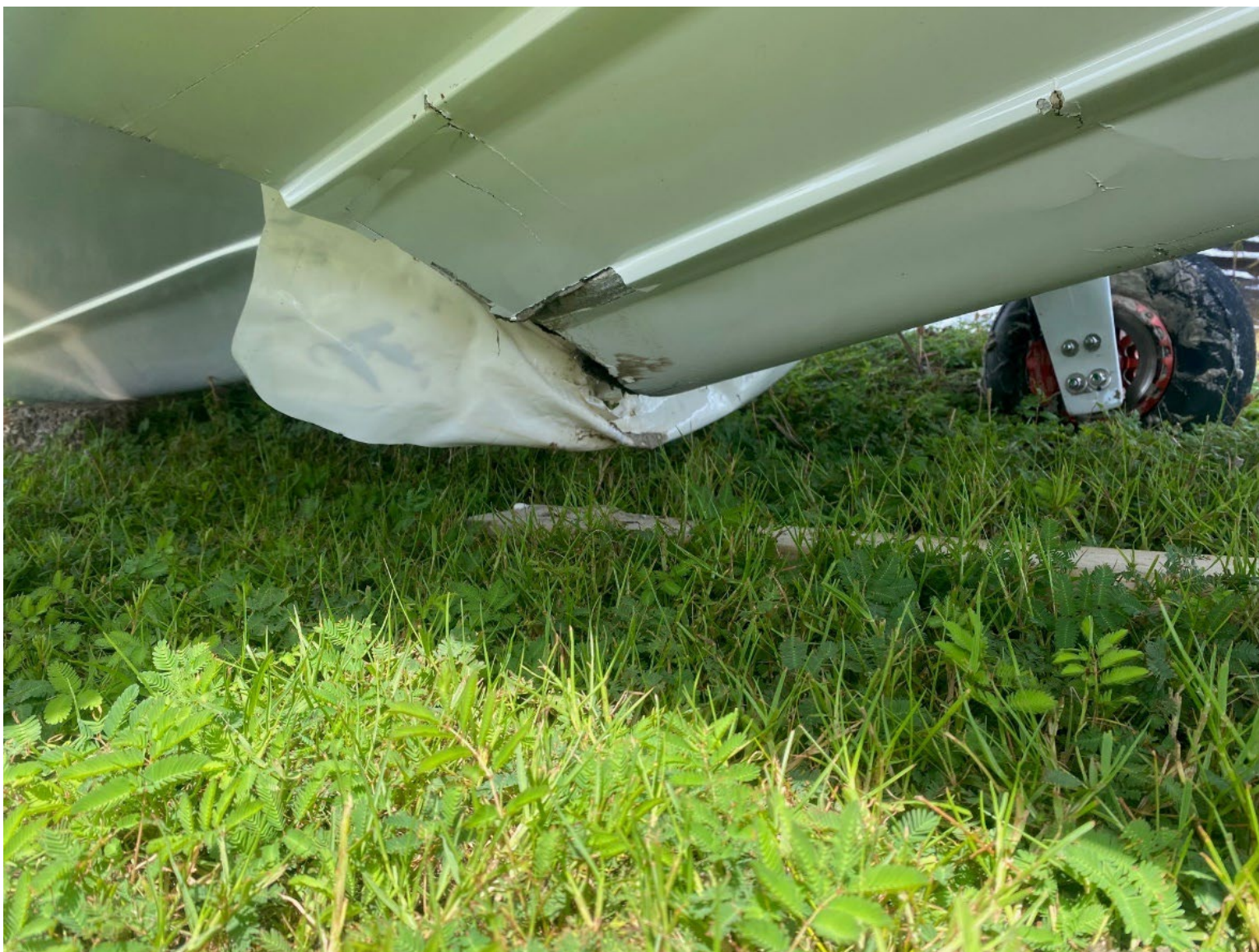
Photograph 1 - View of damage to the fuselage/hull. (Courtesy of FAA)
