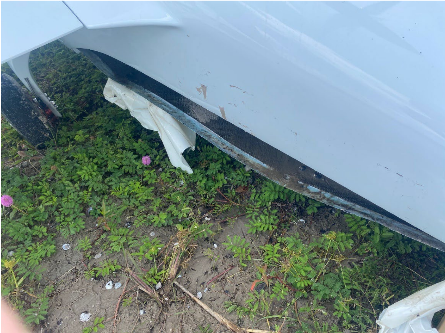
Photograph 2 - View of damage to the left side of the fuselage/hull. (Courtesy of FAA)
