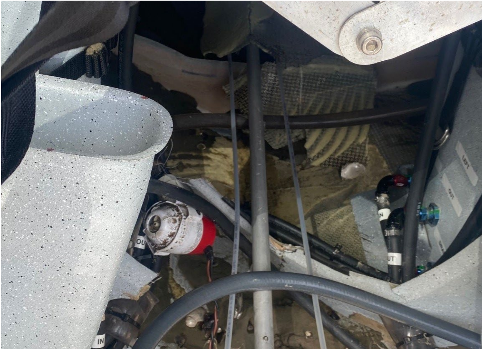
Photograph 3 - View of damage to the internal fuselage/hull structure. (Courtesy of FAA)
