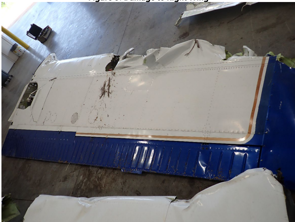
Figure 6: Damage to Left Wing
