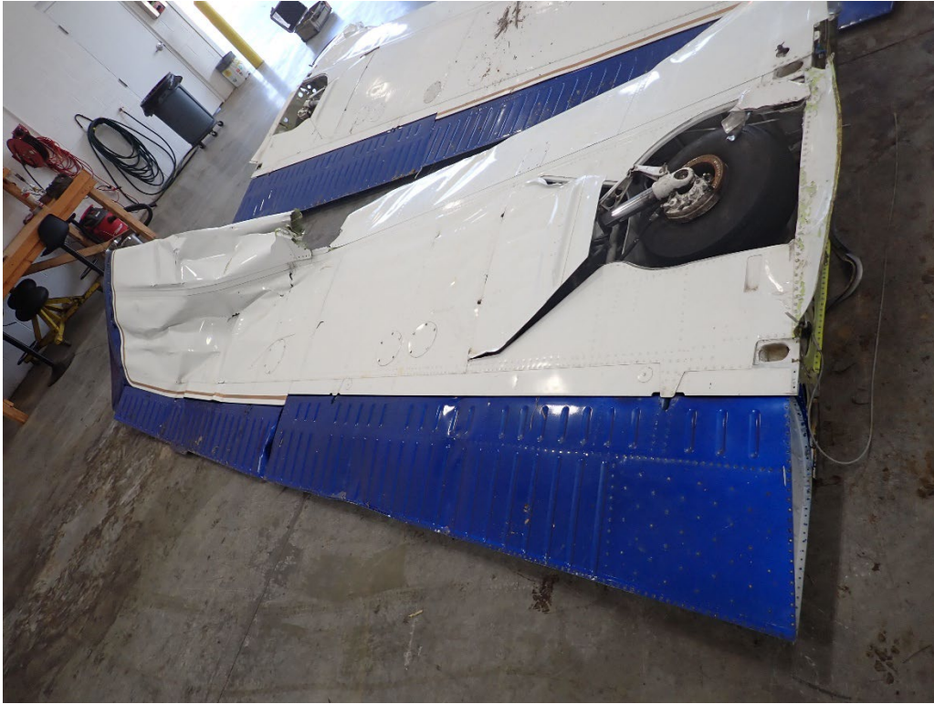
Figure 5: Damage to Right Wing
