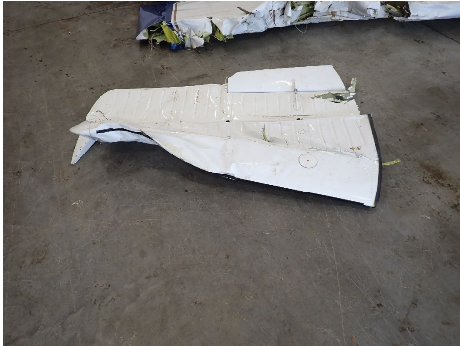
Figure 4: Damage to Right Horizontal Stabilizer
