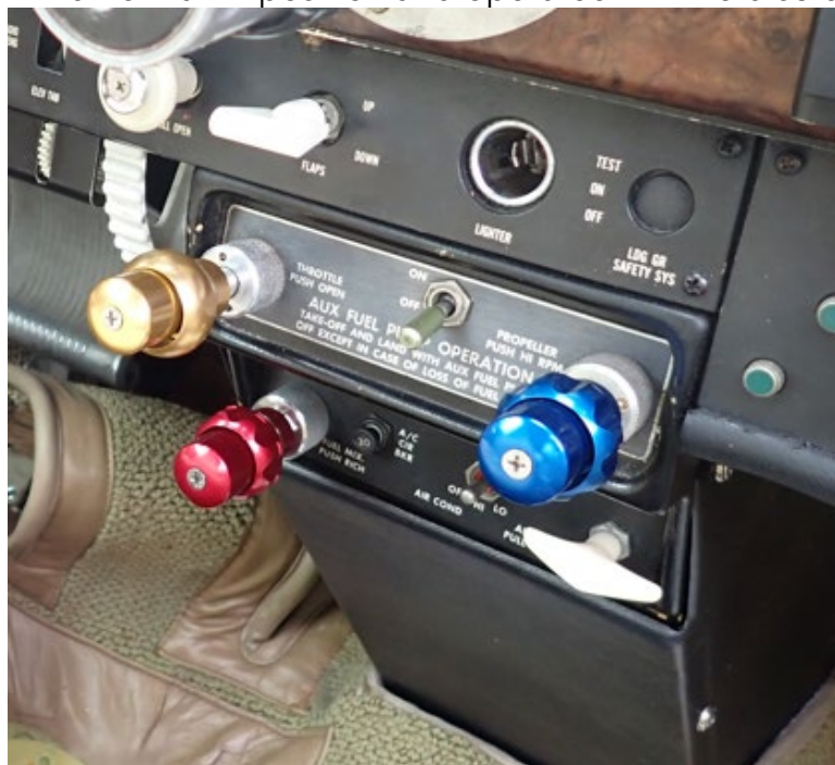
Figure 8: Aux Fuel Switch
