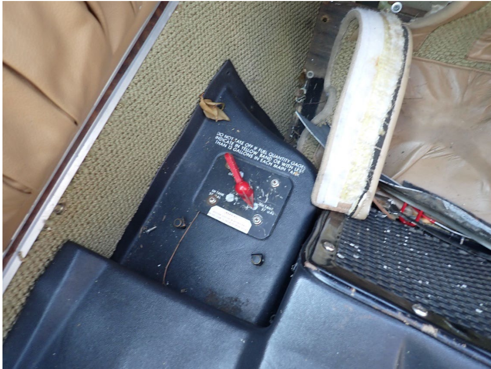
Figure 9: Fuel Selector in Right Tank Position
