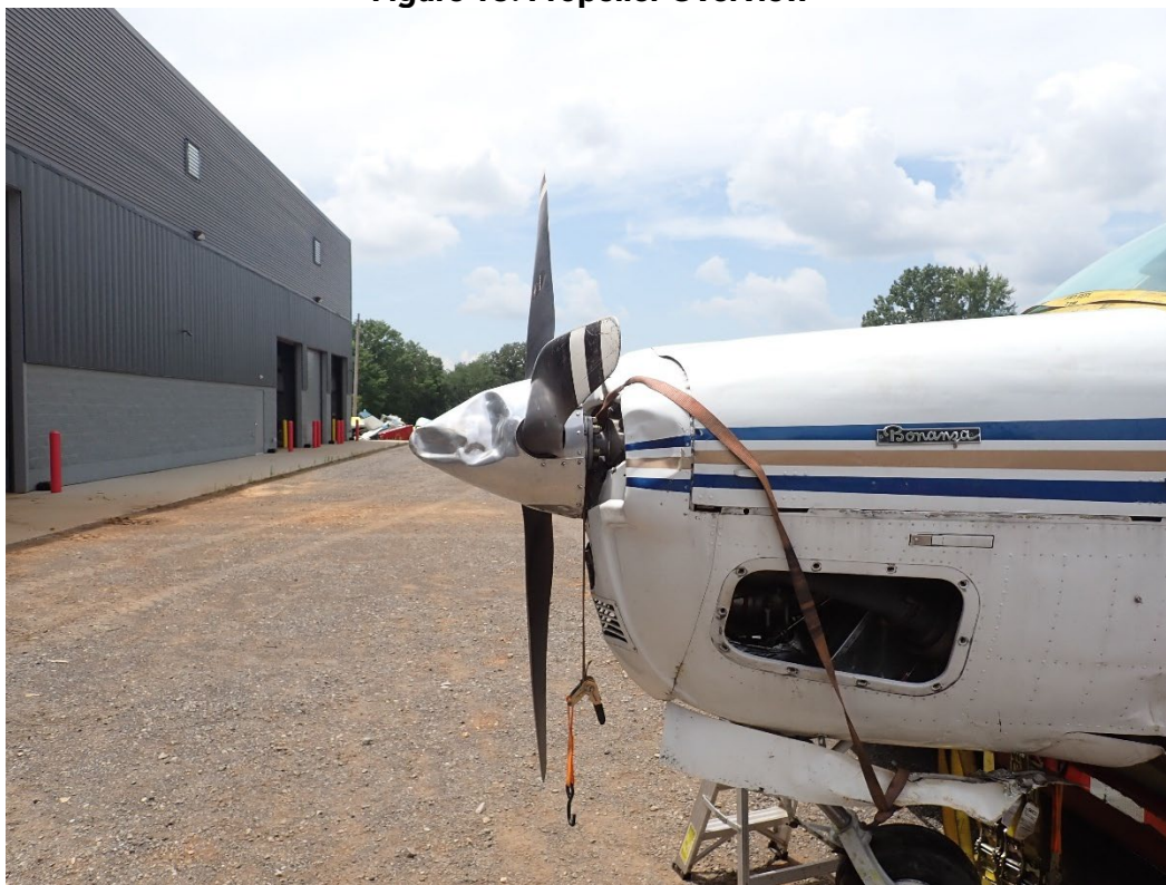
Figure 14: Damage to Propeller Blade
