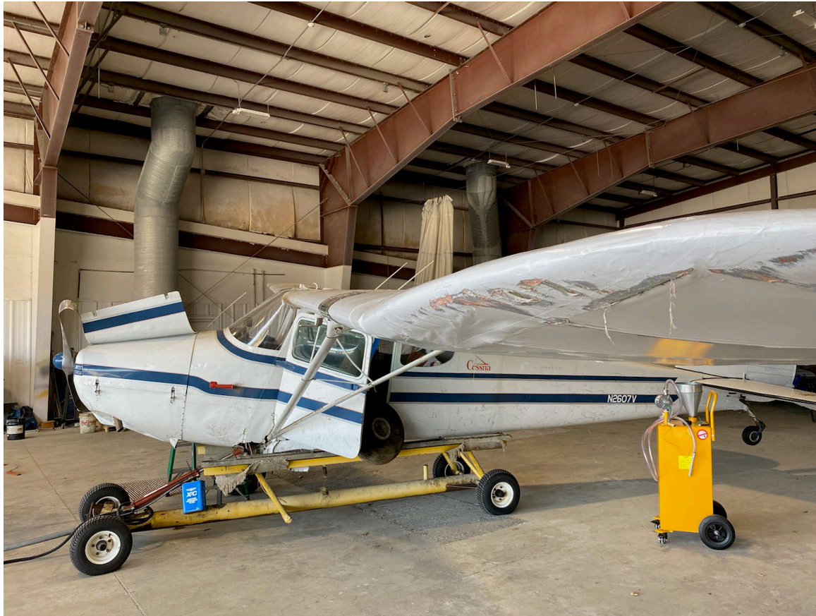
Photograph 1 - Fuselage structure left wing deformation (Courtesy of FAA)
