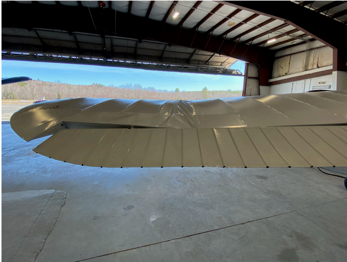
Photograph 2 - Deformation noted to the left wing (Courtesy of FAA)
