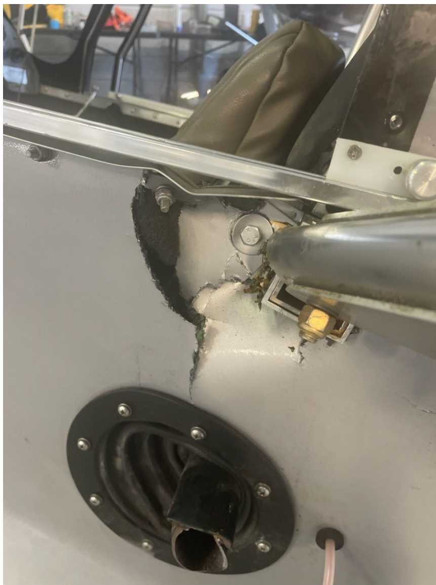
Photograph 2 - Fuselage Damage (Courtesy of FAA)
