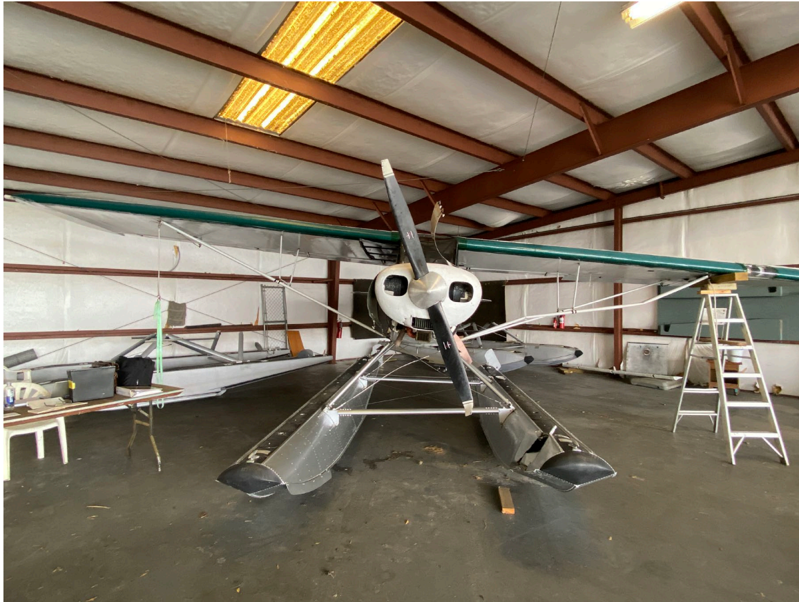
Photograph 1 - Airplane postaccident with damaged wing struts (Courtesy of flight school)
