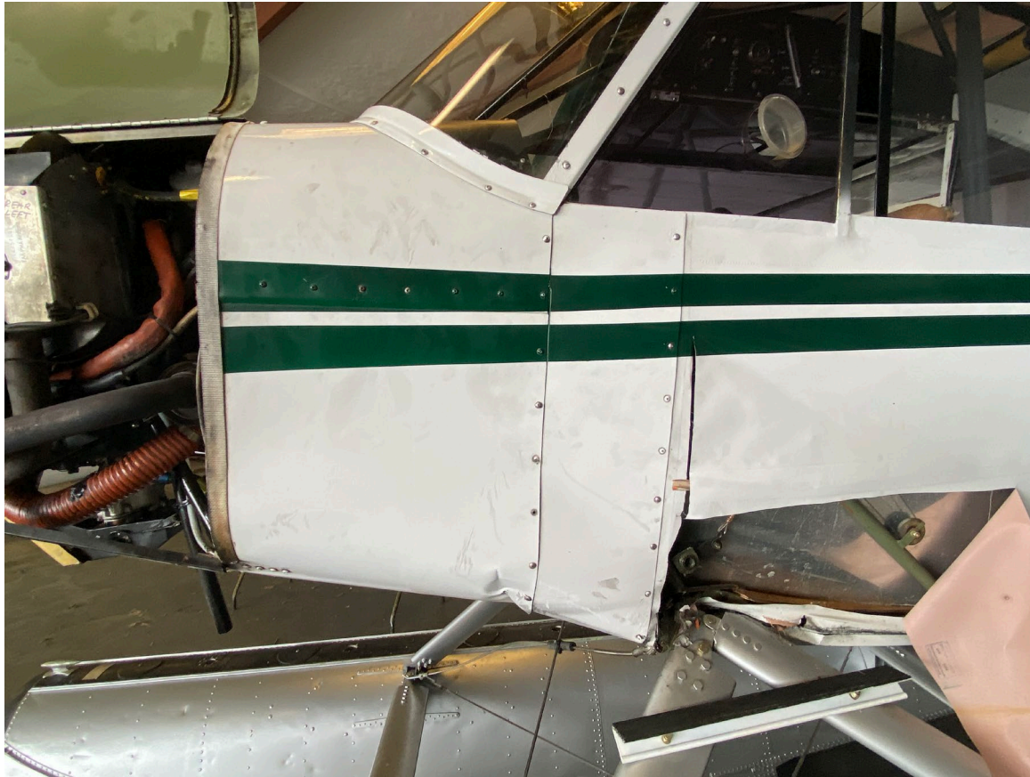
Photograph 3 - Wing strut attach fitting accident damage (Courtesy of flight school)
