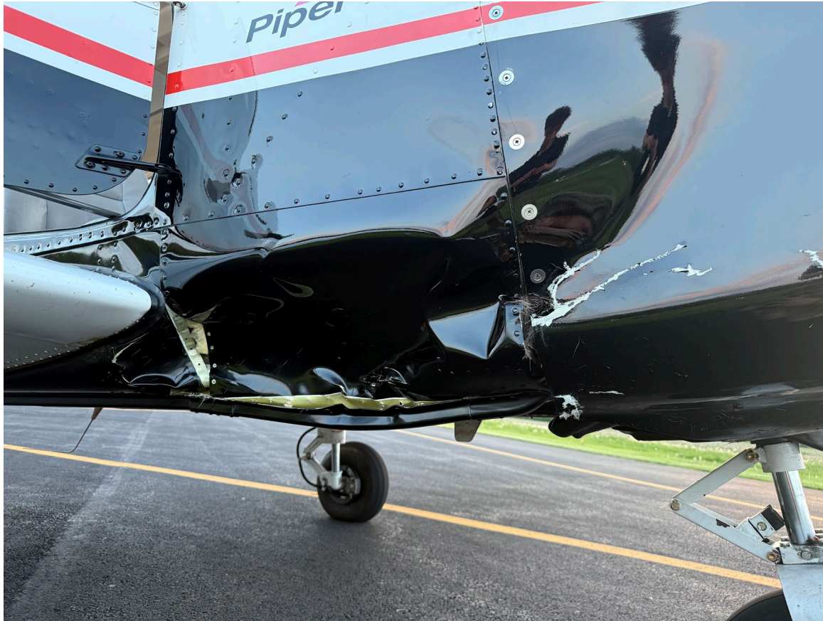
Photograph 1 - Deformation noted to primary structure of fuselage (Courtesy of FAA)
