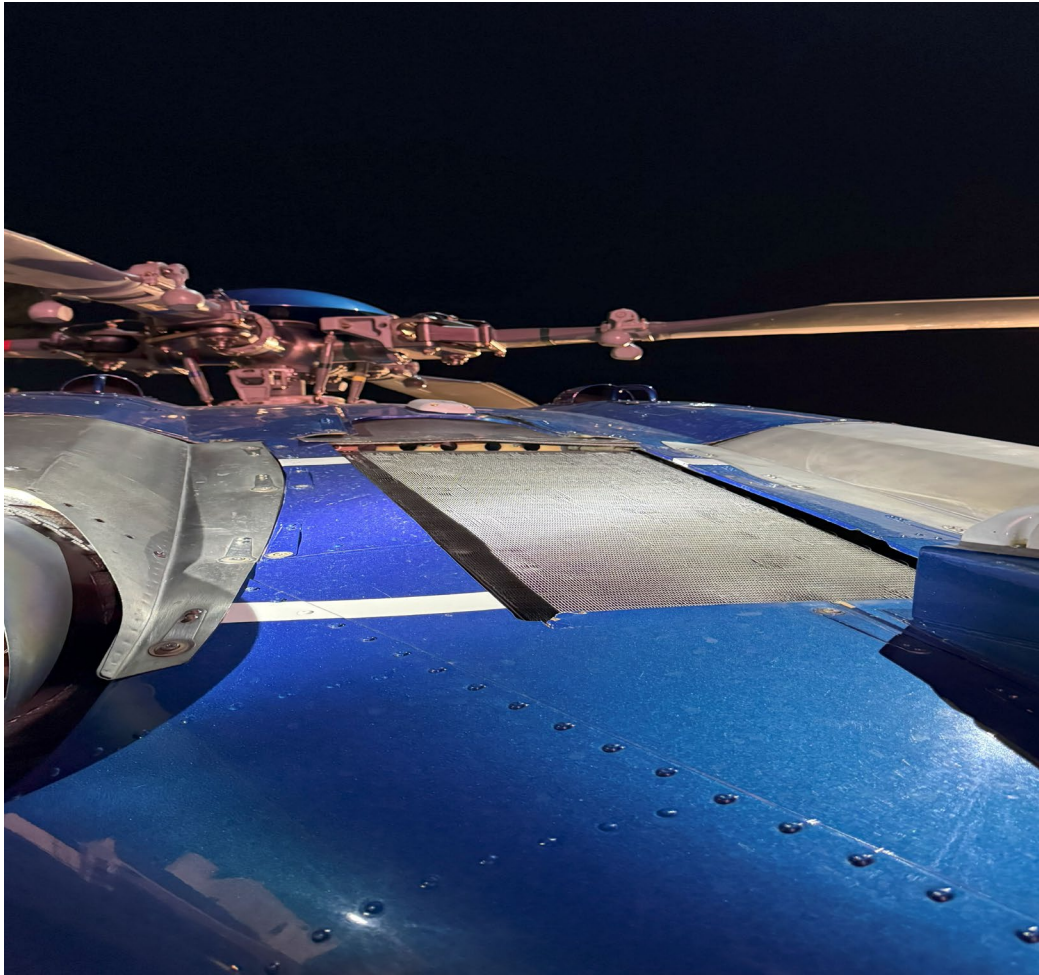
Photograph 4 - View of missing A/C panel (Courtesy of FAA)
