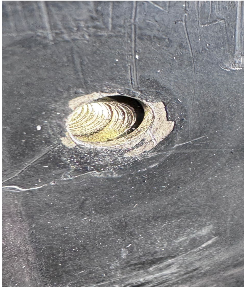
Photograph 7 - View of striped rivnut threads (Courtesy of FAA)
