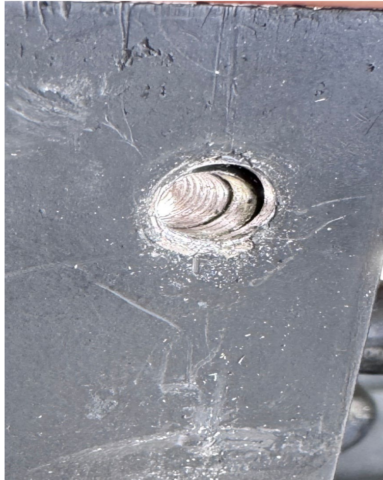
Photograph 6 - View of striped rivnut thread (Courtesy of FAA)
