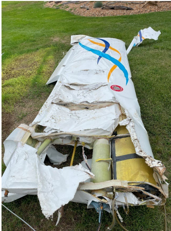
Figure 3, View of impact separated left wing.
