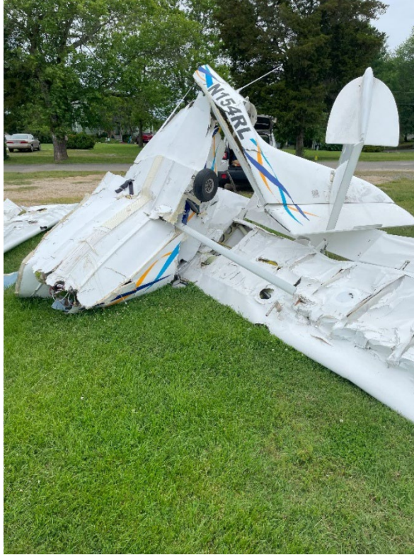
Figure 2, View of right wing, elevator, rudder and bottom of hull.
